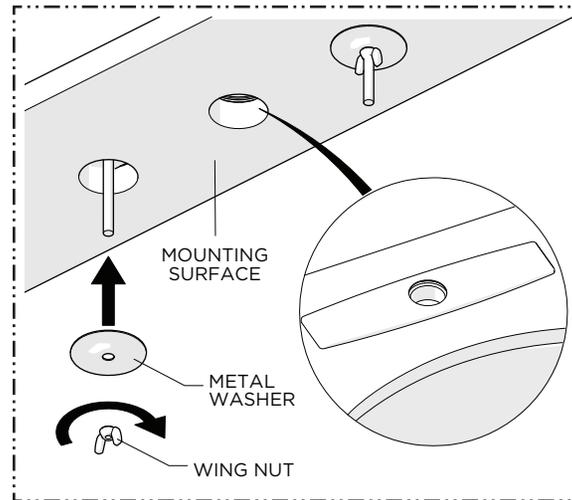
3. Attach the **METAL WASHERS** and **WING NUTS** onto the **THREADED RODS** then ensure the **COVER PLATE** is properly aligned and securely tighten the **WING NUTS**.
