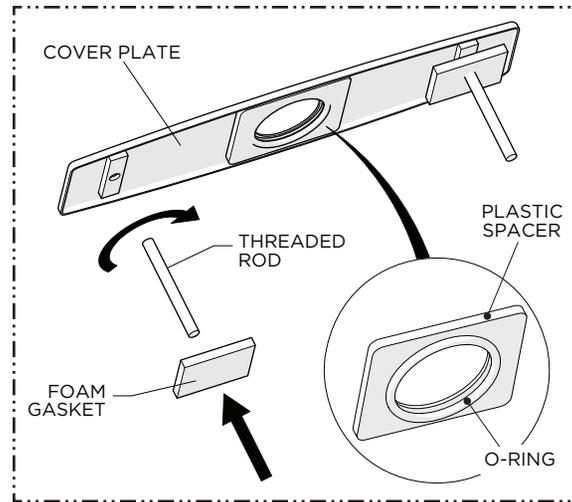
1. Thread the **THREADED RODS** into the **COVER PLATE** then slide the **FOAM GASKETS** onto the **RODS** until they contact the underside of the **PLATE**.
