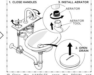
18. Close the HANDLES, open the DRAIN, and re-install the AERATOR.
