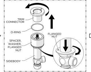
5. Unthread and remove the TRIM CONNECTOR with the O-RING beneath it then fully thread the NUT down the SIDEBODY.
