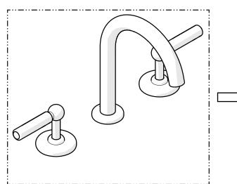
4. Loosen, but do NOT remove the SET SCREW at the base of the ESCUTCHEON then slide the ESCUTCHEON up the HANDLE STEM to expose the RETAINING NUT.
