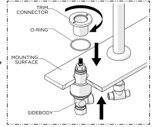
6. Using the O-RING provided, thread the TRIM CONNECTOR back onto the SIDEBODY until it stops then let it rest on the mounting surface.
