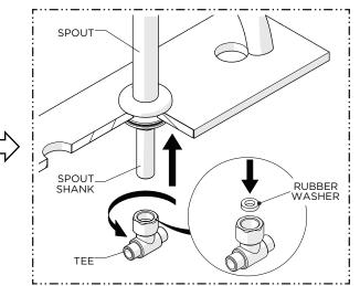
Thread and securely tighten the TEE onto the SHANK making sure to use the RUBBER WASHER provided.
