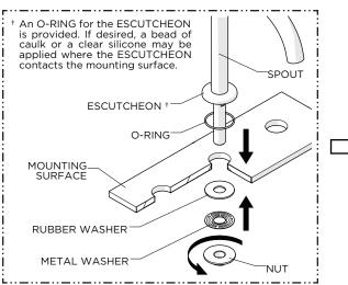
2. Insert the SHANK through the hole on the mounting surface making sure the O-RING provided is beneath the ESCUTCHEON then reattach the RUBBER and METAL WASHERS and securely tighten the NUT.
