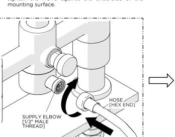
Thread the HEX END of the HOSE to the SUPPLY ELBOW on the VALVE BODY.
