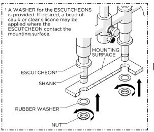
Insert the SHANKS into the holes on the mounting surface then attach the RUBBER and METAL WASHERS and NUTS onto the SHANKS. Securely tighten the NUTS against the underside of the mounting surface.
