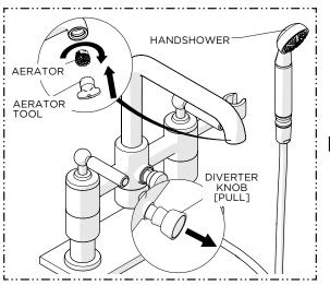
8. With water running, operate the DIVERTER KNOB to ensure it and the HANDSHOWER function properly then turn off the water, and then Re-install the AERATOR.
