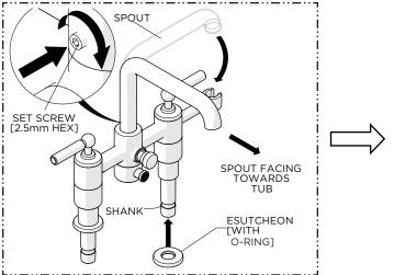
Align the SPOUT properly and securely tighten the SET SCREW at the base of the SPOUT then slide the ESCUTCHEONS onto the SHANKS.
