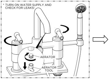
Remove the AERATOR using the TOOL provided then turn on the water supply and operate the HANDLES to flush out the supply lines and check all connections for leaks.
