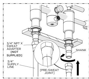
Pre-sweat 3/4" female NPT x sweat adapters to 3/4" supply lines and let cool. Apply a thin coat of pipe thread sealant to the male threads on the SHANKS then thread and securely tighten the ADAPTERS onto the SHANKS.
