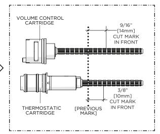
10. Carefully cut the VOLUME CONTROL STEM 9/16" [14mm] in front of the previous mark and THERMOSTATIC STEM 3/8" [10mm] in front of the previous mark so the STEMS will protrude 9/16" [14mm] and 3/8" [10mm] from the finished wall surface respectively.
