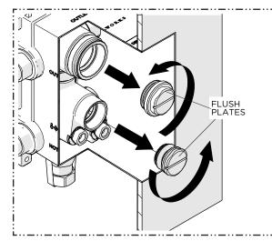
(hot & cold) to flush out the supply lines.
