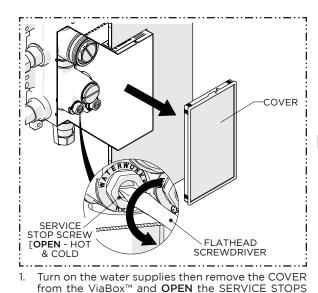
CAUTION: FAILURE TO FLUSH THE SUPPLY LINES WILL PERMANENTLY DAMAGE THE CARTRIDGE AND VOID THE WARRANTY! REPEAT THE FLUSHING PROCESS AS NEEDED BEFORE FINAL TRIM INSTALLATION!
