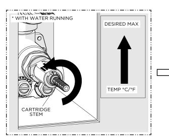
15. Rotate the THERMOSTATIC CARTRIDGE STEM to adjust the temperature to the **maximum** desired bathing temperature, verified with a thermometer, then close the VOLUME CONTROL VALVE and make sure **NOT** to change this setting.
