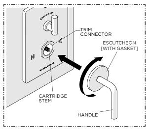
21. With the HANDLE in the desired orientation, place the HANDLE over the CARTRIDGE STEM then thread and securely tighten the ESCUTCHEON into the TRIM CONNECTOR.
