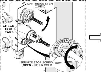
13. OPEN the SERVICE STOPS (hot & cold) and check for leaks. If no leaks are found, turn the CARTRIDGE STEM counterclockwise to open the integrated VOLUME CONTROL VALVE.
