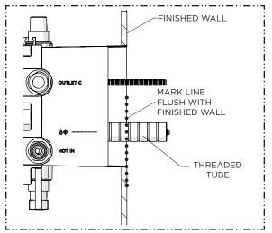
6. Mark the THREADED TUBE where it protrudes past the finished wall.
