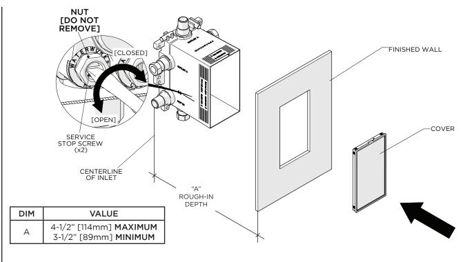
IMPORTANT: The VOLUME CONTROL CARTRIDGE and RETAINING NUT are packaged separately and provided with the VALVE. SET ASIDE UNTIL FINAL TRIM INSTALLATION!
