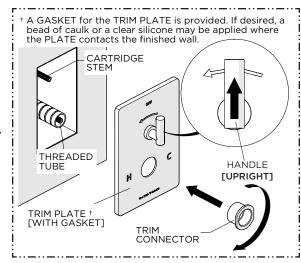
20. With the VOLUME CONTROL HANDLE in an upright vertical position, align the HANDLE with the CARTRIDGE STEM then thread and securely tighten the TRIM CONNECTOR onto the THREADED TUBE.
