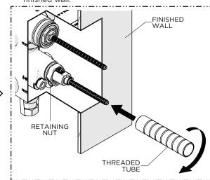
Thread the THREADED TUBE into the THERMOSTATIC RETAINING NUT until snug.
