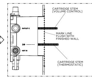
Mark both CARTRIDGE STEMS where they protrude past the finished wall.
