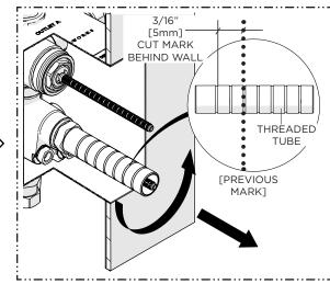
7. Remove the TUBE and cut it 3/16" [5mm] **behind** the previous mark so the TUBE will recess 3/16" [5mm] into the finished wall surface.
