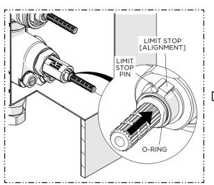
16. Slide the LIMIT STOP and O-RING back down the STEM making sure to properly align the LIMIT STOP with the LIMIT STOP PIN.
