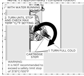
17. Re-open the VOLUME CONTROL VALVE then turn the THERMOSTATIC CARTRIDGE STEM clockwise to full cold then counterclockwise until it stops. Verify the maximum desired bathing temperature set in the previous step then turn the water off.
