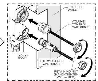
Insert the THERMOSTATIC CARTRIDGE and VOLUME CONTROL CARTRIDGE into the VALVE BODY then thread and hand-tighten the RETAINING NUTS into the VALVE BODY.
