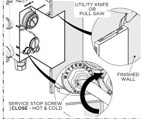
After the lines have been fully flushed, CLOSE the SERVICE STOPS (hot & cold) then, using a utility knife or pull saw, cut the ViaBox™ where it protrudes past the finished wall.
