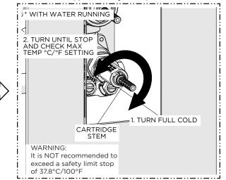
17. Re-open the VOLUME CONTROL VALVE then turn the THERMOSTATIC CARTRIDGE STEM clockwise to full cold then counterclockwise until it stops. Verify the maximum desired bathing temperature set in the previous step then turn the water off. WARNING: It is NOT recommended to exceed a safety limit stop of 37.8°C/100°F.
