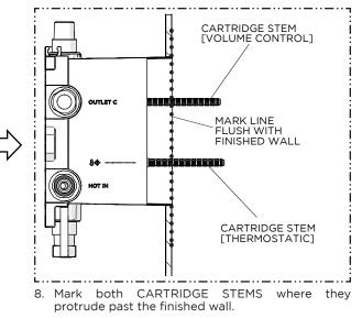
**NOTE:** A straight edge (not supplied) can be used to mark the CARTRIDGE STEMS.
