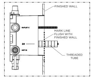
6. Mark the THREADED TUBE where it protrudes past the finished wall.
