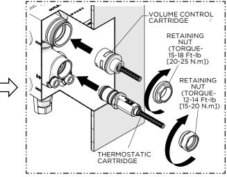
11. Insert both CARTRIDGES back into the VALVE BODY then thread and **securely** tighten the RETAINING NUTS to the specified torque settings shown.
