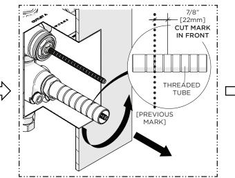
7. Remove the TUBE and cut it 7/8" [22mm] in front of the previous mark so the TUBE will protrude 7/8" [22mm] from the finished wall surface.
