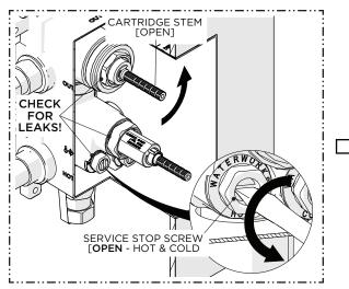
13. **OPEN** both SERVICE STOPS (hot & cold) and check for leaks.
