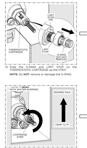
15. Rotate the THERMOSTATIC CARTRIDGE STEM to adjust the temperature to the **maximum** desired bathing temperature, verified with a thermometer, then close the VOLUME CONTROL VALVE and make sure **NOT** to change this setting.
