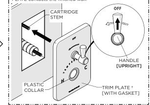
20. With the VOLUME CONTROL HANDLE in an upright vertical position, slide the HANDLE onto the CARTRIDGE STEM.
