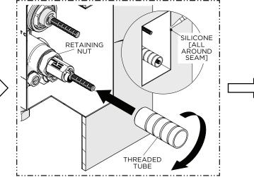
19. Thread the THREADED TUBE back into the RETAINING NUT until snug.
