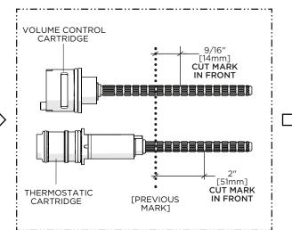
10. Carefully cut the VOLUME CONTROL STEM 9/16" [14mm] in front of the previous mark and THERMOSTATIC STEM 2" [51mm] in front of the previous mark so the STEMS will protrude 9/16" [14mm] and 2" [51mm] from the finished wall surface respectively.
