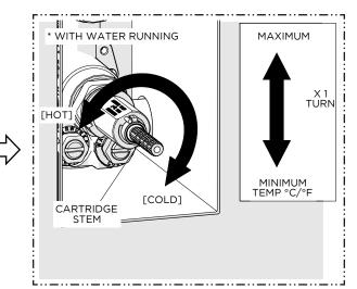
14. With water running, slowly rotate the THERMOSTATIC CARTRIDGE STEM clockwise to attain full cold then rotate it counterclockwise to attain full hot. Verify that a full range of temperatures exists.
