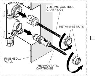
9. Unthread both RETAINING NUTS and remove both CARTRIDGES.
