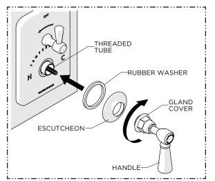
21. Firmly holding the PLATE, RUBBER WASHER, and ESCUTCHEON against the finished wall, thread and securely tighten the GLAND COVER onto the THREADED TUBE.
