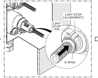
16. Slide the LIMIT STOP and O-RING back down the STEM making sure to properly align the LIMIT STOP with the LIMIT STOP PIN.
