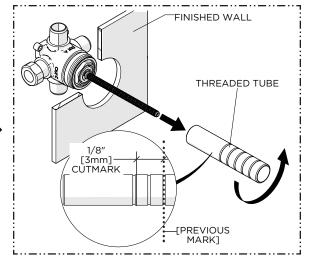
2. Remove the THREADED TUBE then cut it 1/8" [3mm] **behind** the previous mark so the TUBE will recess 1/8" [3mm] into the finished wall surface.
