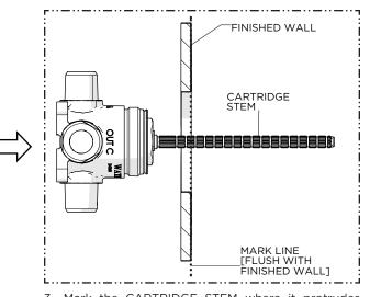
3. Mark the CARTRIDGE STEM where it protrudes past the finished wall.
