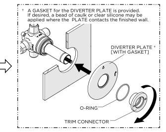
6. Firmly hold the DIVERTER PLATE against the finished wall then thread and securely tighten the TRIM CONNECTOR onto the THREADED TUBE making sure to use the O-RING provided.
