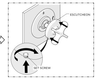
9. CAREFULLY slide the ESCUTCHEON down the HANDLE to conceal the TRIM CONNECTOR, then thread the SET SCREW to secure the position of the ESCUTCHEON.
