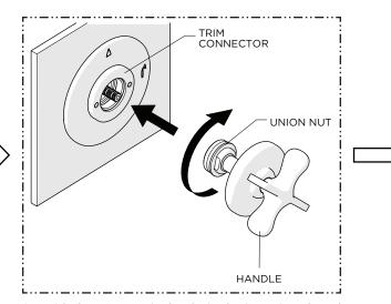
8. With the HANDLE in the desired orientation, thread the UNION NUT into the TRIM CONNECTOR until snug.
