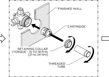
5. Re-insert the CARTRIDGE into the VALVE then thread and securely tighten the RETAINING COLLAR to the specified torgue setting shown.
