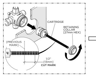
4. Unthread the RETAINING COLLAR and remove the CARTRIDGE then cut the CARTRIDGE STEM 1/2" [13mm] in front of the previous mark so the STEM will protrude 1/2" [13mm] from the finished wall surface.
