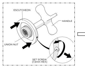
7. Loosen [do **NOT** remove] the SET SCREW at the base of the ESCUTCHEON then **CAREFULLY** slide the ESCUTCHEON up the HANDLE to expose the UNION NUT.
