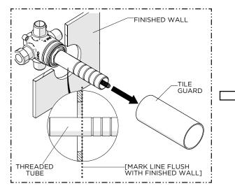
1. Remove the TILE GUARD when ready to install the TRIM then mark the THREADED TUBE where it protrudes past the finished wall.
