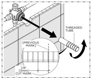
2. Remove the THREADED TUBE then cut it 1/8" [6mm] **behind** the previous mark so the TUBE will recess 1/8" [3mm] into the finished wall surface.
