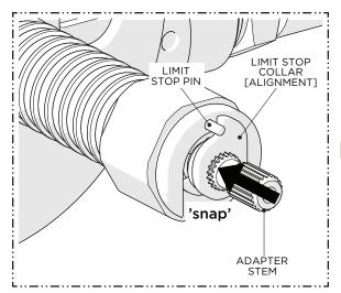
13. Slide the LIMIT STOP COLLAR back down the ADAPTER STEM making sure to properly align it with the LIMIT STOP PIN and press down firmly.
