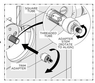
10. Thread the TRIM ADAPTER onto the THREADED TUBE until snug.
