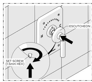
17. CAREFULLY slide the ESCUTCHEON down the HANDLE to conceal the TRIM CONNECTOR, then thread the SET SCREW to secure the position of the ESCUTCHEON.
