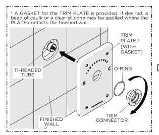
18. Firmly hold the TRIM PLATE against the finished wall then securely tighten the TRIM CONNECTOR onto the THREADED TUBE making sure to use the O-RING provided.
