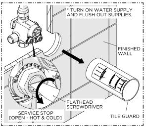
Turn on the water supplies then remove the TILE GUARD from the VALVE and OPEN the SERVICE
