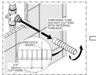
2. Remove the THREADED TUBE then cut it 1/4" [6mm] **behind** the previous mark so the TUBE will recess 1/4" [6mm] into the finished wall surface.
