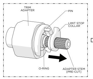
After cutting the ADAPTER STEM, pull the LIMIT STOP COLLAR up the STEM so it no longer contacts the PIN. The COLLAR must be unseated to allow the TRIM ADAPTER to thread properly onto the THREADED TUBE.
