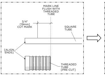
6. Align the pre-cut THREADED TUBE with the SQUARE TUBE then mark and cut the SQUARE TUBE 3/4" [19mm] shorter than the THREADED TUBE.
