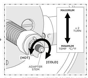
11. Open a **DIVERTER** or **VOLUME CONTROL VALVE** then slowly rotate the ADAPTER STEM clockwise to attain full cold then rotate it counter-clockwise to attain full hot. Verify that a full range of temperatures exists.
