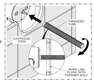
Fully thread the THREADED TUBE [M20] onto the CARTRIDGE STEM and mark the TUBE where it protrudes past the finished wall.
