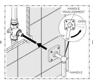
8. Remove and replace the HANDLE to position it as close as possible to the "OFF" position then turn the HANDLE a 1/4 turn to the "OPEN" position making sure NOT to unthread the CARTRIDGE.
