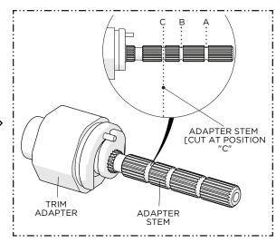
Before installing the TRIM ADAPTER, cut the ADAPTER STEM at position "C" as shown.
