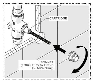
10. Remove the HANDLE then thread and securely tighten the BONNET back onto the CARTRIDGE.
