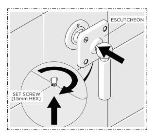
13. CAREFULLY slide the ESCUTCHEON down the HANDLE to conceal the TRIM CONNECTOR, then thread the SET SCREW to secure the position of the ESCUTCHEON.
