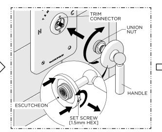
19. Loosen [do NOT remove] the SET SCREW at the base of the ESCUTCHEON then CAREFULLY slide the ESCUTCHEON up the HANDLE to expose the UNION NUT.
