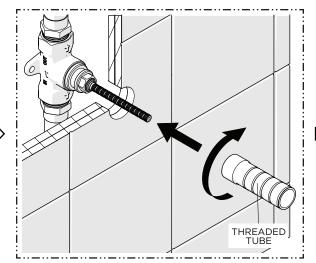
11. Thread and securely tighten the THREADED TUBE back onto the CARTRIDGE until snug.
