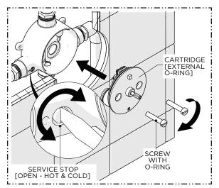
3. Insert the CARTRIDGE into the VALVE BODY then thread and securely tighten the SCREWS, re-open the SERVICE STOPS, and check for leaks.
