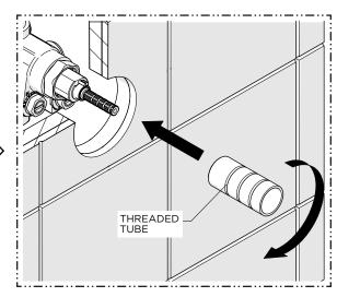
17. Thread the THREADED TUBE back into the RETAINING NUT until snug.
