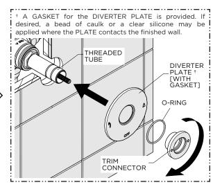
Firmly hold the DIVERTER PLATE against the finished wall then thread and securely tighten the TRIM CONNECTOR onto the THREADED TUBE making sure to use the O-RING provided.
