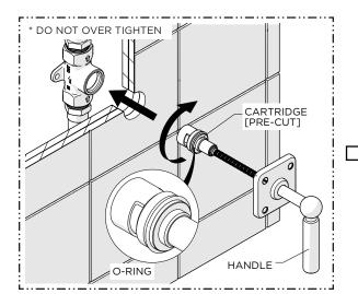
Using the HANDLE, thread the CARTRIDGE back into the VALVE until there is NOTICEABLE resistance.
