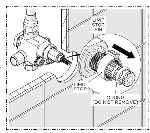
11. Slide the O-RING and LIMIT STOP on the THERMOSTATIC CARTRIDGE up the STEM.
