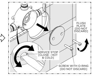
After the lines have been fully flushed, CLOSE the hot and cold SERVICE STOPS then unthread the SCREWS and remove the FLUSH PLATE.
