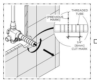
6. Remove the THREADED TUBE then cut it 1/4" [6mm] **in front** of the previous mark so the TUBE will protrude 1/4" [6mm] from the finished wall surface.
