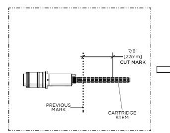
9. Carefully cut the CARTRIDGE STEM 7/8" [22mm] in front of the previous mark so the STEM will protrude 7/8" [22mm] from the finished wall surface.
