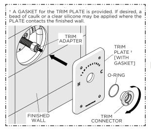
15. Firmly hold the TRIM PLATE against the finished wall then securely tighten the TRIM CONNECTOR onto the TRIM ADAPTER making sure to use the O-RING provided.
