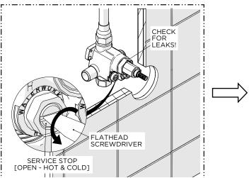
12. Open the SERVICE STOPS (hot & cold) and check for leaks.
