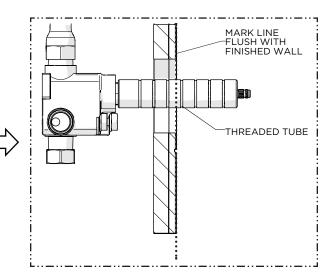
5. Mark the THREADED TUBE where it protrudes past the finished wall.
