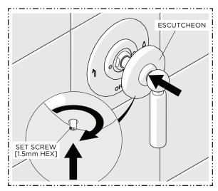
CAREFULLY slide the ESCUTCHEON down the HANDLE to conceal the TRIM CONNECTOR, then thread the SET SCREW to secure the position of the ESCUTCHEON.
