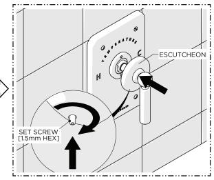
20. CAREFULLY slide the ESCUTCHEON down the HANDLE to conceal the TRIM CONNECTOR, then thread the SET SCREW to secure the position of the ESCUTCHEON.
