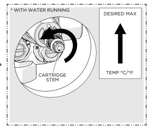
14. With water running, rotate the CARTRIDGE STEM to adjust the temperature to the **maximum** desired bathing temperature, verified with a thermometer, then turn the water off and make sure **NOT** to change this setting.
