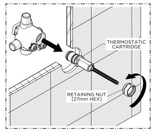
8. Unthread the RETAINING NUT and remove the CARTRIDGE.
