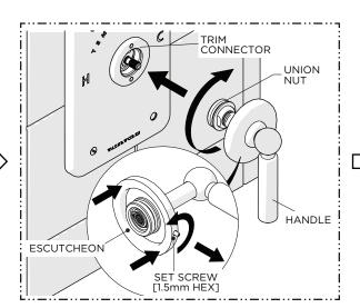
16. Loosen [do NOT remove] the SET SCREW at the base of the ESCUTCHEON then CAREFULLY slide the ESCUTCHEON up the HANDLE to expose the UNION NUT
