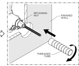
4. Thread the THREADED TUBE [M24] into the RETAINING NUT until it stops.
