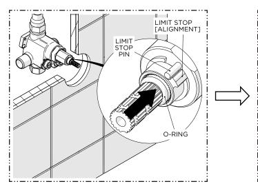
15. Slide the LIMIT STOP and O-RING back down the STEM making sure to properly align the LIMIT STOP with the LIMIT STOP PIN.
