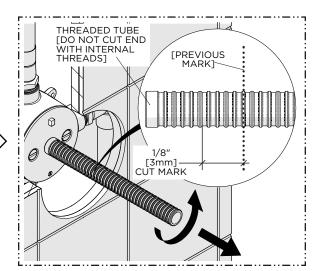
5. Remove the THREADED TUBE then cut it 1/8" [3mm] behind the previous mark.
