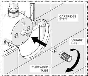
Slide the SQUARE TUBE onto the CARTRIDGE STEM then thread the THREADED TUBE onto the STEM until snug.
