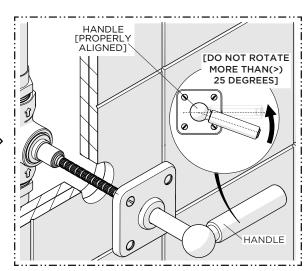
If needed, carefully continue to rotate the HANDLE counter-clockwise to obtain the proper alignment.
