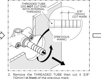
CAUTION: Do NOT cut the end with the internal threads.
