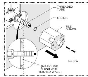
Remove the TILE GUARD when ready to install the TRIM then mark the THREADED TUBE where it protrudes past the finished wall.
