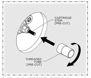
9. Thread the THREADED TUBE back onto the CARTRIDGE until it stops.
