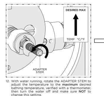
CAUTION: IF THE MAXIMUM BATHING TEMPERATURE IS NOT CORRECT OR NEEDS TO BE ADJUSTED, SLIGHTLY PULL THE LIMIT STOP COLLAR FORWARD SO [ IT DOES NOT HIT THE PIN AND REPEAT STEPS 11 THROUGH 14 TO RE-CALIBRATE THE TEMPERATURE SETTING.
