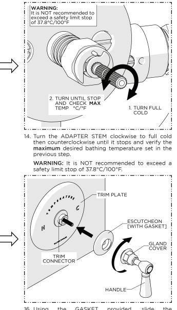
16. Using the GASKET provided, slide the ESCUTCHEON over the TRIM CONNECTOR then thread and securely tighten the GLAND COVER onto the TRIM CONNECTOR.
