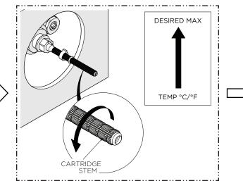
5. With water running, rotate the CARTRIDGE STEM to adjust the temperature to the **maximum** desired bathing temperature, verified with a thermometer, then turn the water off and make sure **NOT** to change this setting.
