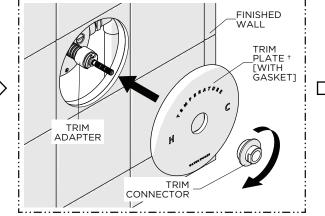
15. Firmly hold the TRIM PLATE against the finished wall then thread and securely tighten the TRIM CONNECTOR onto the TRIM ADAPTER.
