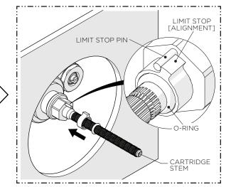
6. Slide the LIMIT STOP and O-RING back down the CARTRIDGE STEM making sure to properly align the LIMIT STOP with the LIMIT STOP PIN.
