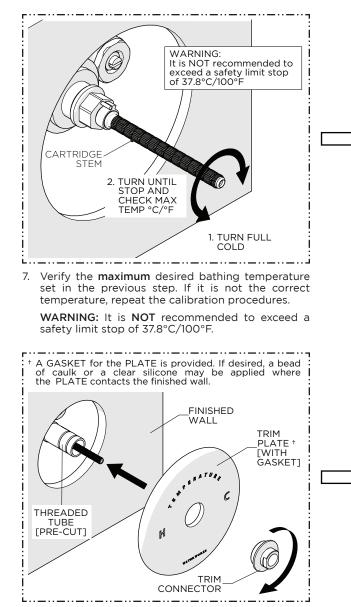
10. Firmly hold the TRIM PLATE against the finished wall then thread and securely tighten the TRIM CONNECTOR onto the THREADED TUBE.
