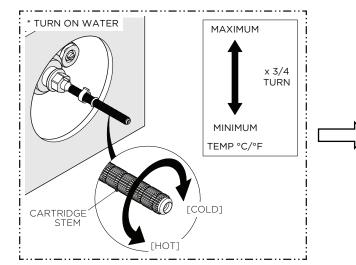
4. Turn on the water supply and open a DIVERTER or VOLUME CONTROL VALVE then slowly rotate the CARTRIDGE STEM clockwise to attain full cold then rotate it counterclockwise to attain full hot. Verify that a full range of temperatures exists.
