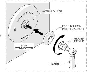
11. Using the GASKET provided, slide the ESCUTCHEON over the TRIM CONNECTOR then thread and securely tighten the GLAND COVER onto the TRIM CONNECTOR.
