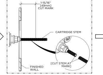
8. Mark the CARTRIDGE STEM 1-15/16" [49mm] in front of the finished wall then cut the STEM at the marked location.
