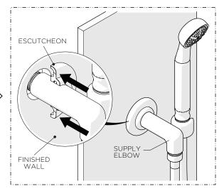
Slide the ESCUTCHEON up the ELBOW until it contacts the finished wall.
