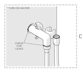
Turn on the water and a diverter/wall valve (sold separately) to flush out any debris in the supply line and inspect all connections for leaks then turn the water off.
