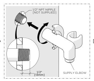
Ensure the 1/2" NPT NIPPLE (not supplied) projects 1/2" [13mm] from the surface of the finished wall then thread and securely tighten the SUPPLY ELBOW onto the NIPPLE.
