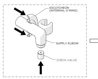
1. Slide the ESCUTCHEON onto the SUPPLY ELBOW.
