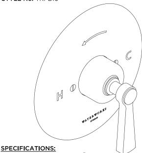
Rough-in Depth Minimum: 1\%" Rough-in Depth Maximum: 2\%" Integrated Diverter: No
