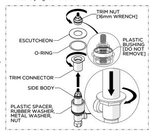
Unthread and remove the TRIM NUT, remove the ESCUTCHEON with the O-RING, unthread and remove the TRIM CONNECTOR then fully thread the NUT down the SIDEBODY.
