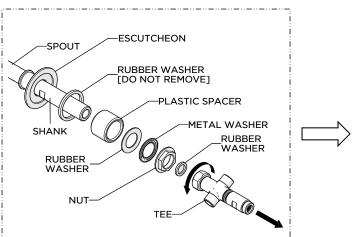
Unthread and remove the TEE, NUT, lower deck WASHERS and PLASTIC SPACER from SHANK.
