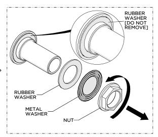
Unthread and remove the NUT, METAL WASHER, and RUBBER WASHER from the SHANK.
