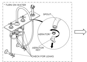
16. Unthread and remove the AERATOR then turn on the water to flush out any debris in the supply lines and inspect all connections for leaks.
