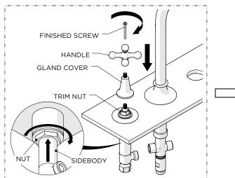
Re-attach the GLAND COVER, HANDLE and FINISHED SCREW. Ensure the HANDLE is in the desired orientation then securely tighten the NUT on the SIDEBODY
