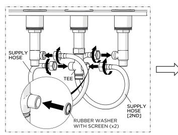
Connect the SIDEBODIES to the TEE using the SUPPLY HOSES provided. Securely tighten the HOSES and ensure they are not pinched/kinked.
