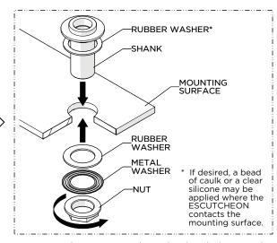
12. Insert the SHANK through the hole on the mounting surface making sure the RUBBER WASHER provided is beneath the ESCUTCHEON then re-install the WASHERS and securely tighten the NUT.
