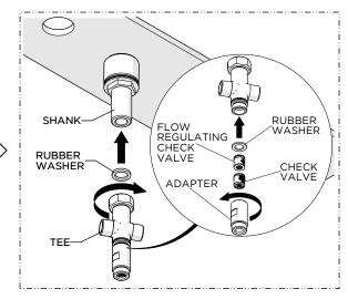
3. Using the RUBBER WASHER provided, thread and securely tighten the TEE back onto the SHANK.
