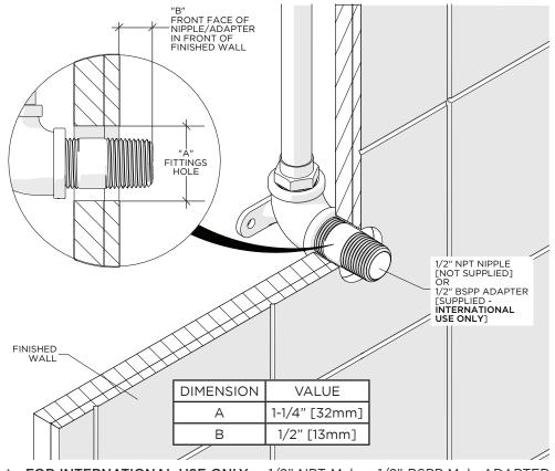
**FOR INTERNATIONAL USE ONLY**, a 1/2" NPT Male x 1/2" BSPP Male ADAPTER (Style No. UNUK04) is provided. The BSPP end of the ADAPTER may be field cut.
