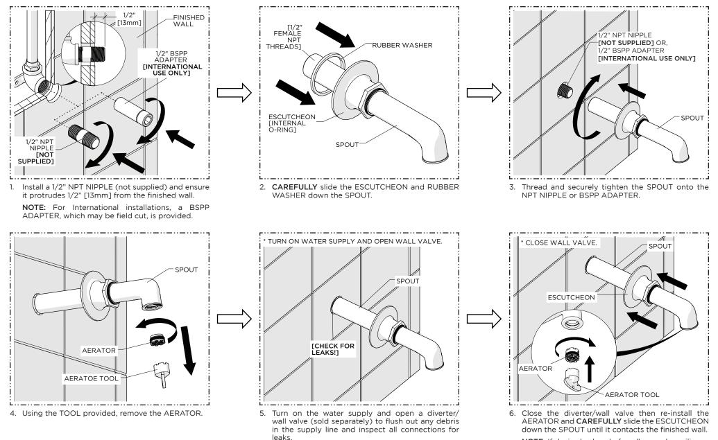
**NOTE:** If desired, a bead of caulk or a clear silicone may be applied where the ESCUTCHEON contacts the finished wall.
