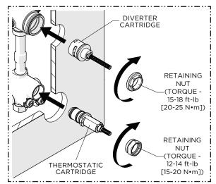
Insert both CARTRIDGES back into the VALVE BODY then thread and securely tighten the RETAINING NUTS to the specified torque settings shown.
