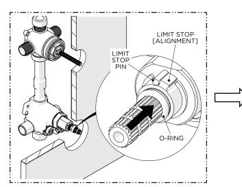
15. Slide the LIMIT STOP and O-RING back down the STEM making sure to properly align the LIMIT STOP with the LIMIT STOP PIN.
