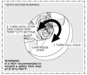
16. Re-open the DIVERTER VALVE then turn the THERMOSTATIC CARTRIDGE STEM clockwise to full cold then counterclockwise until snug. Verify the maximum desired bathing temperature set in the previous step then turn the water off.
