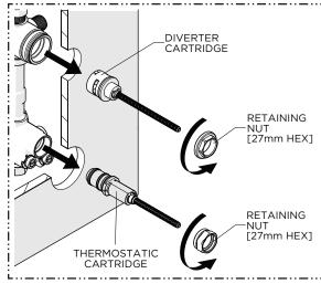
Unthread both RETAINING NUTS and remove both CARTRIDGES.
