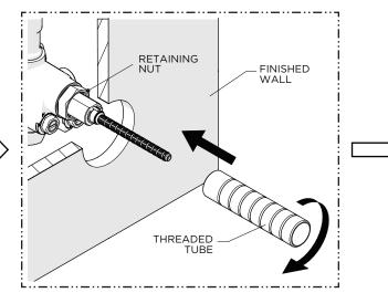
4. Thread the THREADED TUBE into the RETAINING NUT until snug.
