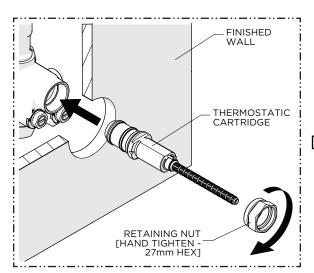
Insert the THERMOSTATIC CARTRIDGE into the VALVE BODY then thread and hand-tighten the RETAINING NUT into the VALVE BODY.
