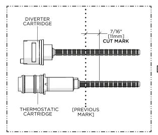
Carefully cut both CARTRIDGE STEMS 7/16" [11mm] in front of the previous mark so the STEMS will protrude 7/16" [11mm] from the finished wall surface.
