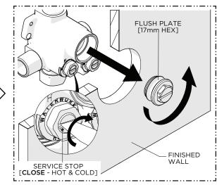
After the lines have been fully flushed, CLOSE the SERVICE STOPS (hot & cold) then unthread and remove the FLUSH PLATE.
