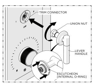
22. **CAREFULLY** slide the ESCUTCHEON up the LEVER HANDLE to expose the UNION NUT then thread the NUT into the TRIM CONNECTOR until snug.
