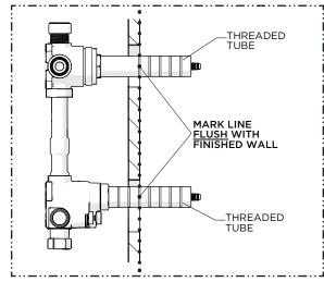
Mark both TUBES where they protrude past the finished wall.
