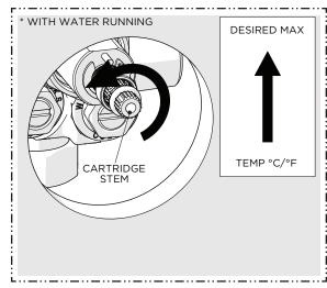
14. With water running, rotate the STEM to adjust the temperature to the **maximum** desired bathing temperature, verified with a thermometer, then close the DIVERTER VALVE and make sure **NOT** to change this setting.
