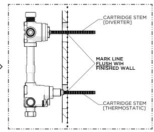
7. Mark both CARTRIDGE STEMS where they protrude past the finished wall.
