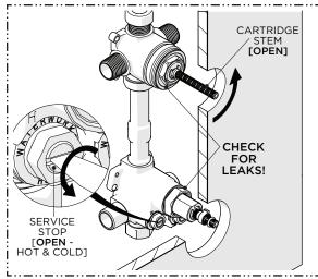
12. **OPEN** the SERVICE STOPS (hot & cold) and check for leaks. If no leaks are found, proceed and open the INTEGRATED DIVERTER VALVE
