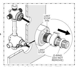
11. Slide the O-RING and LIMIT STOP on the THERMOSTATIC CARTRIDGE up the STEM.
