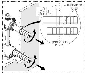
Remove the TUBES and cut them 1/8" [3mm] behind the previous mark so the TUBES will be 1/8" [3mm] below or recessed into the finished wall surface.
