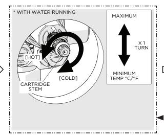
13. With water running, slowly rotate the THERMOSTATIC CARTRIDGE STEM clockwise to attain full cold then rotate it counterclockwise to attain full hot. Verify that a full range of temperatures exists.
