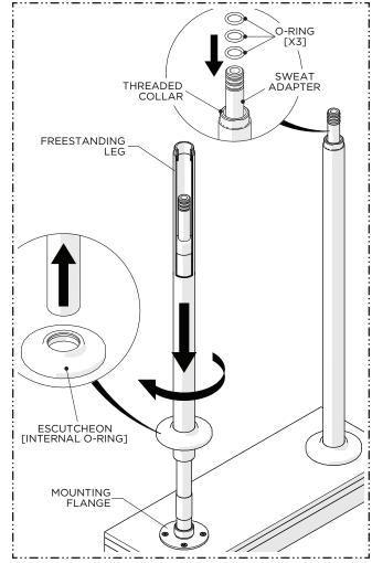
4. Slide the ESCUTCHEONS onto the FREESTANDING LEGS then slide the LEGS over the SUPPLY LINES and thread them onto the MOUNTING PLATES. Re-attach the O-RINGS onto the SWEAT ADAPTERS.
