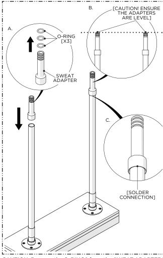
CAUTION: Remove the O-RINGS from the SWEAT ADAPTERS prior to soldering to prevent damaging them.
