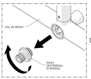
Unthread and remove the POST from the VALVE BODY
