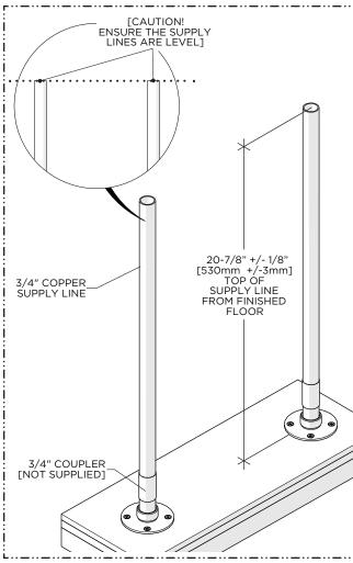
2. Using 3/4" COUPLERS (not supplied), extend the supply lines to 20-7/8" +/- 1/8" [530mm +/- 3mm] above the finished floor.
