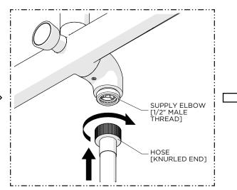
8. Thread the KNURLED END of the HOSE to the SUPPLY ELBOW on the VALVE BODY.
