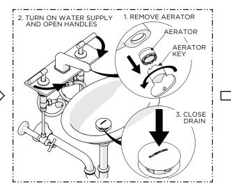
18. Remove the AERATOR, turn on the water supply and open the HANDLES to flush out the supply lines, and inspect all connections for leaks then close the DRAIN to ensure it functions properly.
