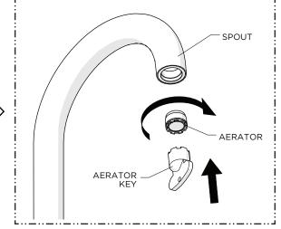
17. Re-install the AERATOR using the tool provided.
