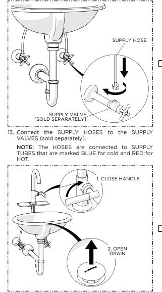
16. Close the HANDLE then open the DRAIN to drain the water.
