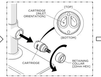
2. Unthread and remove the RETAINING COLLAR then pull the CARTRIDGE out.
