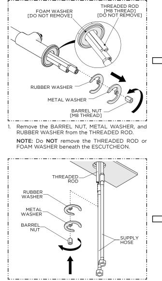
4. Slide the RUBBER and METAL WASHERS back onto the THREADED ROD then thread and securely tighten the BARREL NUT onto the ROD.
