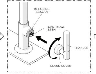
5. With the HANDLE held vertically, thread the GLAND COVER onto the RETAINING COLLAR until snug.
