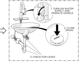
15. Turn on the water supply and operate the HANDLE to flush out the supply lines. Inspect all connections for leaks then close the DRAIN to ensure it functions properly.
