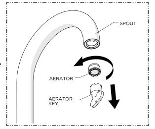
Remove the AERATOR from the SPOUT using the AERATOR KEY provided.
