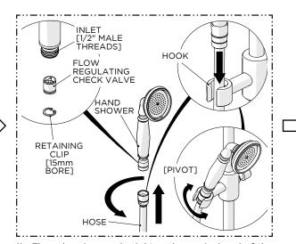
Thread and securely tighten the conical end of the HOSE to the HANDSHOWER then place it into the HOOK and pivot the HANDSHOWER to the desired position.
