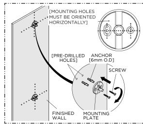
6. Using the previous marks as a reference, install the MOUNTING PLATES using the ANCHORS, if necessary, and SCREWS provided.
