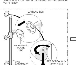
5. Loosen, but do NOT remove, the SET SCREW on each BAR END and remove the MOUNTING PLATES.
