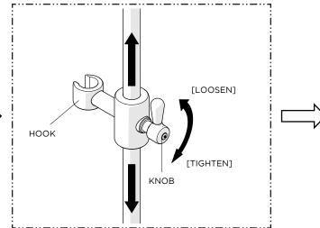
8. Loosen the KNOB and adjust the HOOK on the BAR ASSEMBLY to the desired height then securely retighten the KNOB.
