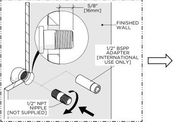
Install a 1/2" NPT NIPPLE (not supplied) and ensure it protrudes 5/8" [16mm] from the finished wall.
