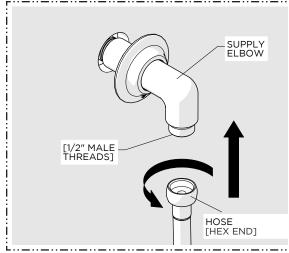
Thread and securely tighten the HEX END of the HOSE to the SUPPY ELBOW.
