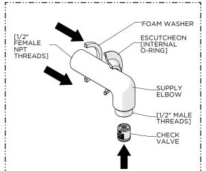
Slide the ESCUTCHEON and FOAM WASHER down the SUPPLY ELBOW.
