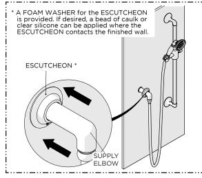
Slide the ESCUTCHEON down the SUPPLY ELBOW until it contacts the finished wall.
