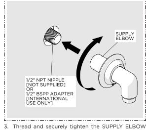
onto the NPT NIPPLE or BSPP ADAPTER.
