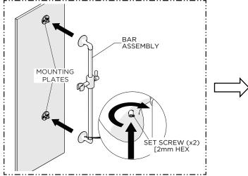
Slide the BAR ASSEMBLY onto the MOUNTING PLATES then thread and securely tighten the SET SCREWS.
