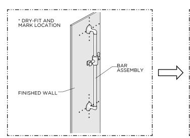
4. Dry-fit the BAR ASSEMBLY to the finished wall and mark the ideal location for installation; preferably over adequate blocking or stud material.
