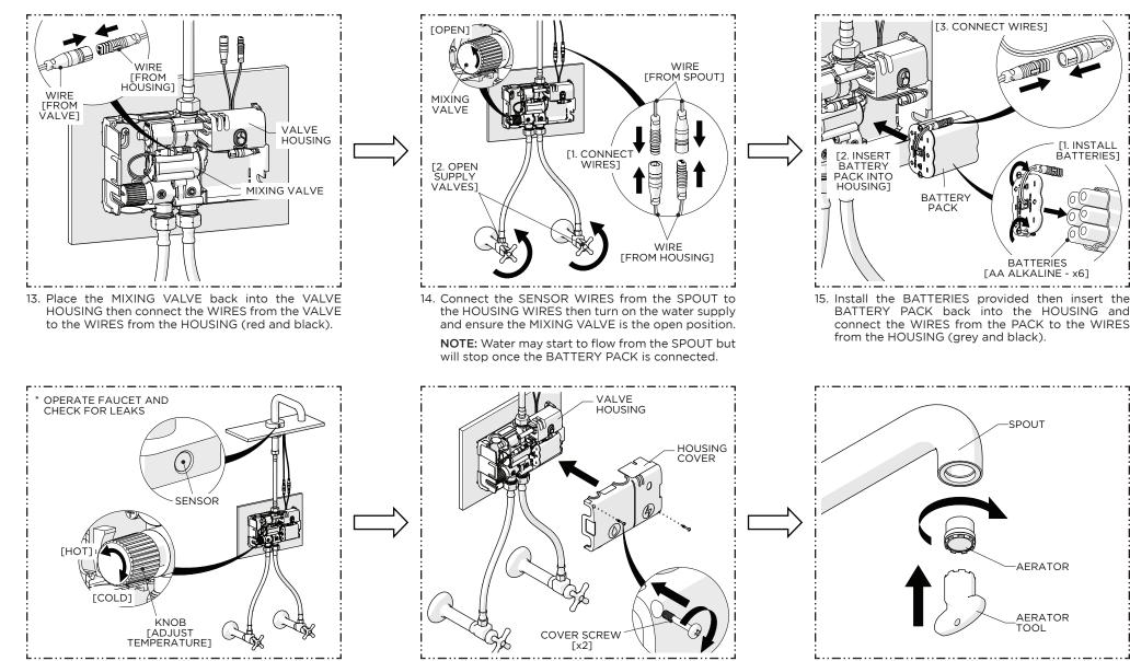
17. Re-attach the HOUSING COVER. 18. Re-install the AERATOR and finish the installation.
