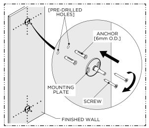
6. Using the previous marks as a reference, install the MOUNTING PLATES using the ANCHORS, if necessary, and SCREWS provided.
