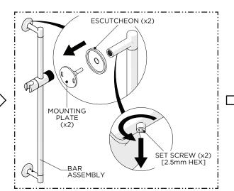
5. Loosen, but do NOT remove, the SET SCREW on each end of the BAR then remove the MOUNTING PLATES and ESCUTCHEONS.
