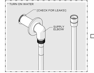
10. Turn on the water and a diverter/wall valve (sold separately) to flush out any debris in the supply line and inspect all connections for leaks then turn the water off.
