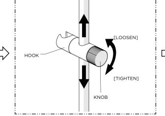
Loosen the KNOB and adjust the HOOK on the BAR ASSEMBLY to the desired height then securely retighten the KNOB.
