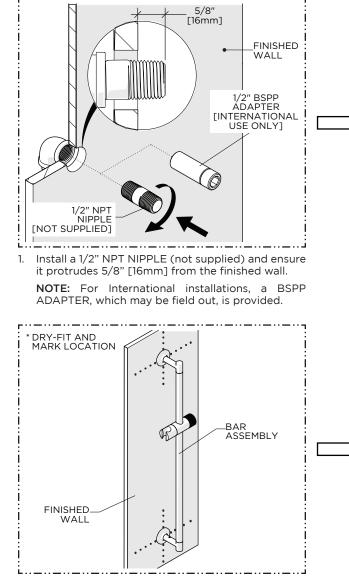
4. Dry-fit the BAR ASSEMBLY to the finished wall and mark the ideal location for installation; preferably over adequate blocking or stud material.
