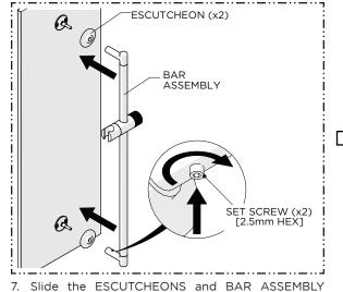
Slide the ESCUTCHEONS and BAR ASSEMBLY onto the MOUNTING PLATES then thread and securely tighten the SET SCREWS.
