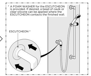
12. Slide the ESCUTCHEON down the SUPPLY ELBOW until it contacts the finished wall.
