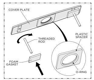
Thread the THREADED RODS into the COVER PLATE then slide the FOAM GASKETS onto the RODS until they contact the underside of the PLATE.
