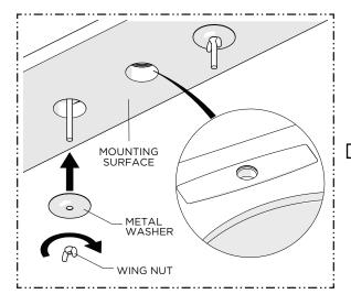
Attach the METAL WASHERS and WING NUTS onto the THREADED RODS then ensure the COVER PLATE is properly aligned and securely tighten the WING NUTS.
