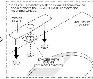
Insert the THREADED RODS into the holes on the mounting surface.
