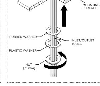
2. Insert the INLET/OUTLET TUBES and SHANK through the hole on the mounting surface. Place HANDLE in off position, line up SPOUT with HANDLE and position SPOUT over sink in desired location then re-attach the WASHERS and securely tighten the NUT.
