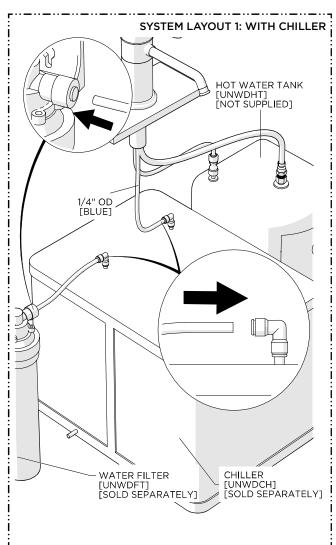
INSTALLING WITH CHILLER (SYSTEM LAYOUT 1) Insert the BLUE 1/4" O.D. TUBE from the SPOUT into the CHILLER [SOLD SEPARATELY] 1/4" OUTLET. Insert "O.D TUBE [SUPPLIED WITH THE FILTER] from the WATER FILTER OUTLET [SOLD SEPARATELY] into the CHILLER INLET.
