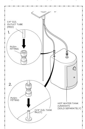
Insert the RED 1/4" O.D. OUTLET TUBE from the SPOUT into the PUSH-FITTING then connect the FITTING to the 1/4" O.D. TANK INLET.
