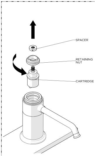
Remove the SPACER then unthread the RETAINING NUT and remove the CARTRIDGE.
