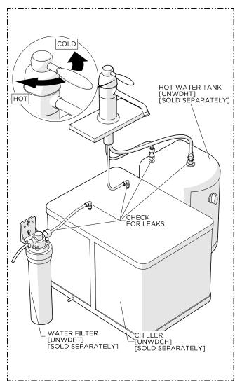
7. Turn on the water to flush out any debris in the supply lines, operate the HANDLE and SPOUT to ensure they function properly and inspect all connection for leaks.
