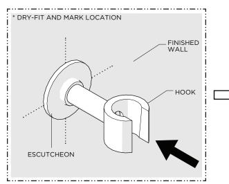
4. Dry-fit the HOOK to the finished wall and mark the ideal location for installation; preferably over adequate blocking or stud material.
