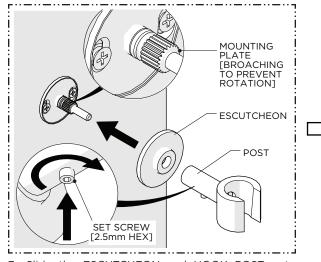
7. Slide the ESCUTCHEON and HOOK POST onto the MOUNTING PLATE then thread and securely tighten the SET SCREW.
