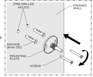
6. Using the previous marks as a reference, install the MOUNTING PLATE using the ANCHORS, if necessary, and SCREWS provided.
