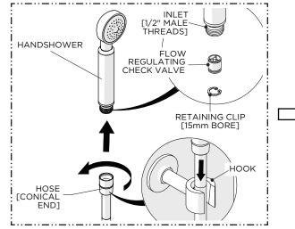
10. Thread and securely tighten the conical end of the HOSE to the HANDSHOWER then place it into the HOOK.
