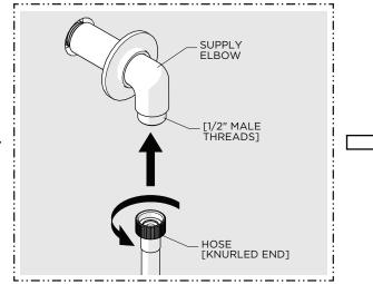
Thread and securely tighten the KNURLED end of the HOSE to the ELBOW.
