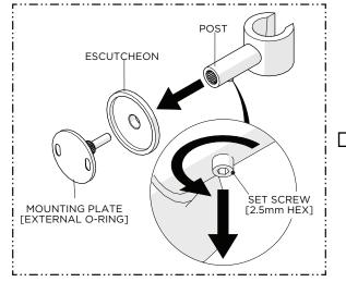
5. Loosen, but do NOT remove, the SET SCREW on the HOOK POST then remove the MOUNTING PLATE and ESCUTCHEON.
