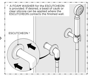
11. Slide the ESCUTCHEON down the SUPPLY ELBOW until it contacts the finished wall.
