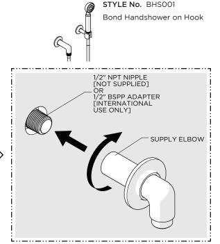
3. Thread and securely tighten the SUPPLY ELBOW onto the NPT NIPPLE or BSPP ADAPTER.
