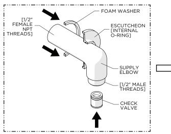
Slide the ESCUTCHEON and FOAM WASHER down the SUPPLY ELBOW.
