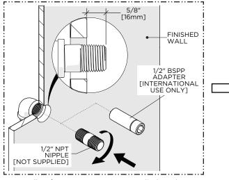
. Install a 1/2" NPT NIPPLE (not supplied) and ensure it protrudes 5/8" [16mm] from the finished wall.
