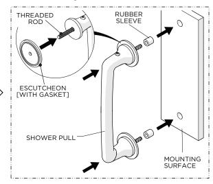
Insert the RUBBER SLEEVES into the pre-drilled holes then slide the ESCUTCHEONS over the THREADED RODS on the PULL and insert the RODS through the RUBBER SLEEVES.
