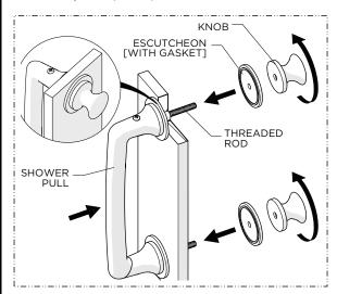
While holding the PULL against the mounting surface, slide the ESCUTCHEONS onto the THREADED RODS then thread and securely tighten the KNOBS onto the RODS.
