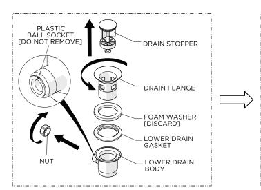
Unthread and remove the DRAIN STOPPER, DRAIN FLANGE, LOWER DRAIN GASKET, and NUT from the LOWER DRAIN BODY.
