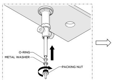
7. Insert the O-RING and METAL WASHER into the base of the TEE then thread and securely tighten the PACKING NUT.
