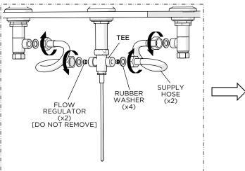
14. Connect the SIDEBODIES to the TEE using the SUPPLY HOSES and RUBBER WASHERS provided. Securely tighten the HOSES and ensure they are not pinched/kinked.
