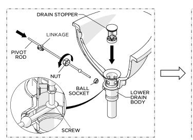
19. Making sure the BALL SOCKET is in place, insert the PIVOT ROD into the DRAIN BODY and securely tighten the NUT then insert the STOPPER into the FLANGE making sure the SCREW rests on top of the PIVOT ROD. Adjust the SCREW if needed.
