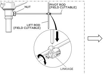
20. Connect the LIFT ROD to the PIVOT ROD using the LINKAGE provided.
