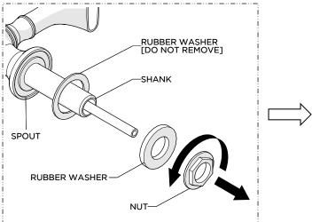
2. Unthread and remove the NUT and lower deck WASHER from the SHANK.
