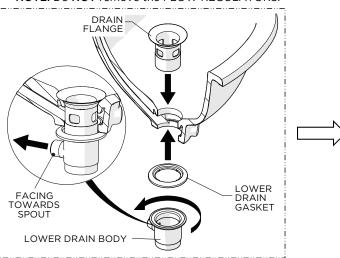
17. Set the DRAIN FLANGE into the lavatory (sold separately) using putty or a clear silicone and attach the LOWER DRAIN GASKET then securely tighten the LOWER DRAIN BODY onto the FLANGE.
