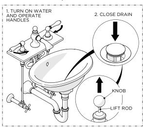
22. Turn on the water to flush out the supply lines and inspect all connections for leaks then close the DRAIN to ensure it functions properly. Turn off and drain the water.
