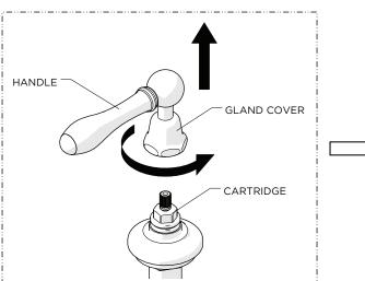
8. Unthread the GLAND COVER from the CARTRIDGE on the SIDEBODY and pull the HANDLE off.
