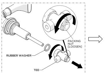
Loosen, but do NOT remove the PACKING NUT at the base of the TEE then remove the TEE and RUBBER WASHER from the SHANK.
