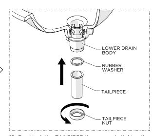
18. Re-attach the TAILPIECE then securely tighten the NUT onto the LOWER DRAIN BODY making sure to include the RUBBER WASHER provided.
