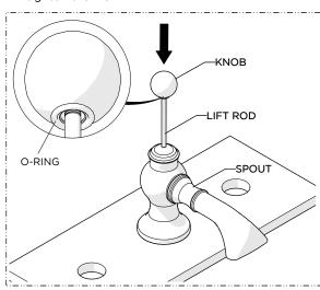
Insert the LIFT ROD into the top of the SPOUT making sure the O-RING is beneath the KNOB.
