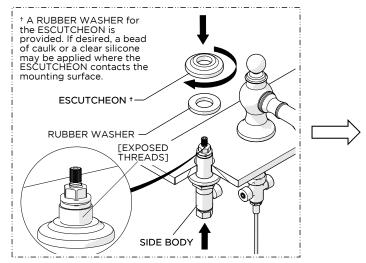
10. Using the RUBBER WASHER provided, thread the ESCUTCHEON back onto the SIDEBODY and let it rest on the mounting surface.
