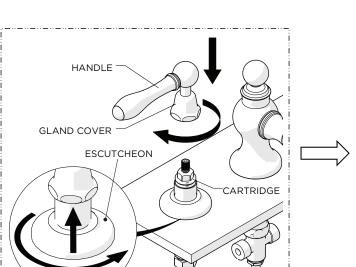
11. With the HANDLE in the desired orientation, thread the GLAND COVER back onto the CARTRIDGE until it stops then unthread the ESCUTCHEON until it contacts the GLAND COVER.
