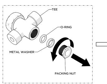
4. Remove the PACKING NUT, METAL WSAHER and O-RING from the TEE to prevent the GUIDE TUBE in the SPOUT from damaging the O-RING.
