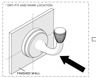
1. Dry-fit the product to the finished wall and mark the ideal location for installation.
