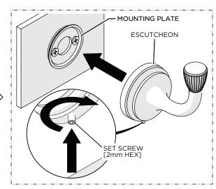
Place the product over the MOUNTING PLATE and securely tighten the SET SCREW.
