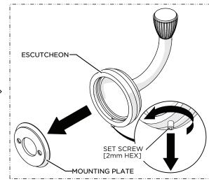
Loosen, but do <u>NOT</u> remove, the SET SCREW on the bottom of ESCUTCHEON using a 2mm HEX KEY and remove the MOUNTING PLATE.
