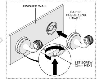
4. Place both PAPER HOLDER ENDS over the MOUNTING PLATES and securely tighten the SET SCREWS using a 2mm HEX KEY.
