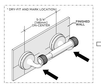
1. Dry-fit the product to the finished wall and mark the ideal location making sure to hold the product level.
