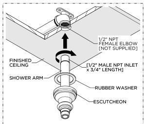
Making sure the ELBOW (not supplied) is properly roughed-in, thread and securely tighten the SHOWER ARM into the ELBOW.
