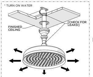
5. Turn on the water and operate the SHOWER HEAD to ensure it pivots and functions properly. Inspect all connections for leaks then turn the water off.
