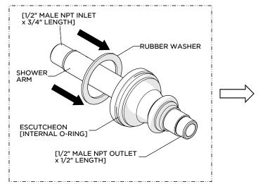
Slide the ESCUTCHEON and RUBBER WASHER onto the SHOWER ARM.
