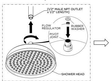
Insert the RUBBER WASHER into the PIVOT JOINT on the SHOWER HEAD then thread and securely tighten the PIVOT JOINT onto the SHOWER ARM.
