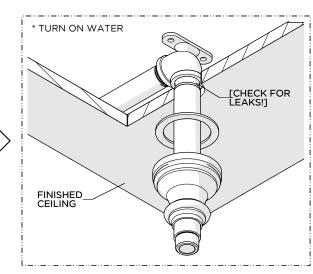
Turn on the water and a diverter/wall valve (sold separately) to flush out any debris in the supply line and inspect all connections for leaks then turn the water off.
