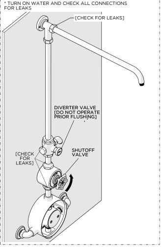
9. Turn on the water and operate the SHUTOFF VALVE to flush out the supply lines, check all connections for leaks then turn the water off.
