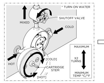
16. Turn on the water and open the SHUTOFF VALVE then slowly rotate the CARTRIDGE STEM clockwise to attain full cold then counterclockwise to attain full hot. It's approximately 2 complete rotations. Verify a full range of temperatures exists.
