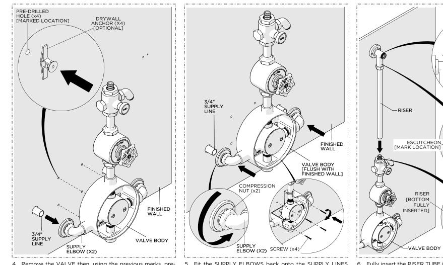
4. Remove the VALVE then, using the previous marks, predrill the holes (pilot holes) to accommodate the 1-1/2" WOOD SCREWS and, if necessary, install the DRYWALL ANCHORS provided where blocking is not installed.
