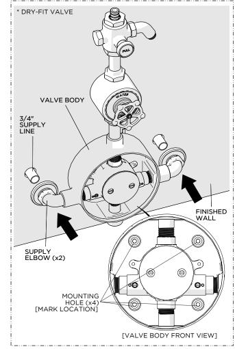
3. Fit the SUPPLY ELBOWS onto the SUPPLY LINES making sure the VALVE BODY sits flush against the finished wall then mark the location of the MOUNTING HOLES (x4).
