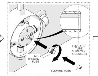
17. **FULLY** thread the ALL THREAD TUBE onto the CARTRDIGE then insert the SQUARE TUBE into the ALL THREAD and onto the CARTRIDGE STEM.
