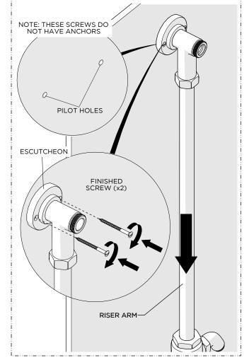
7. Remove the RISER TUBE then, using the previous marks, pre-drill the holes (pilot holes) to accommodate the 2-1/2" FINISHED WOOD SCREWS (x2) provided.
