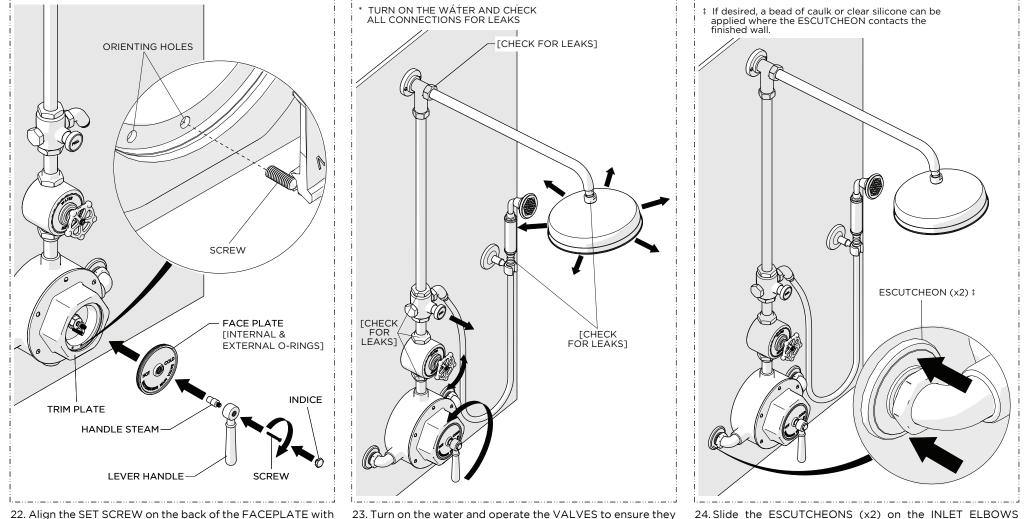
22. Align the SET SCREW on the back of the FACEPLATE with the ALIGNMENT HOLE at 6 o'clock on the TRIM PLATE then push the FACEPLATE into the TRIM PLATE making sure it is fully seated.
