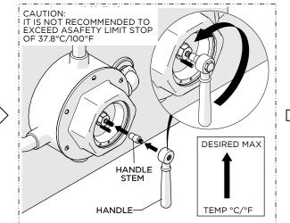
20. With water running, and using the HANDLE STEM and HANDLE adjust the temperature to the <u>MAXIMUM</u> desired bathing temperature, verified with a thermometer. Turn the water off and make sure **NOT** to change this setting.
