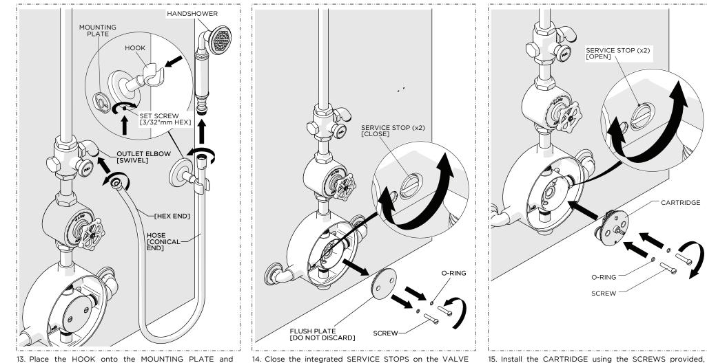
13. Place the HOOK onto the MOUNTING PLATE and securely tighten the SET SCREW then connect the HOSE to the HANDSHOWER and DIVERTER VALVE and place the HANSHOWER on the HOOK.
