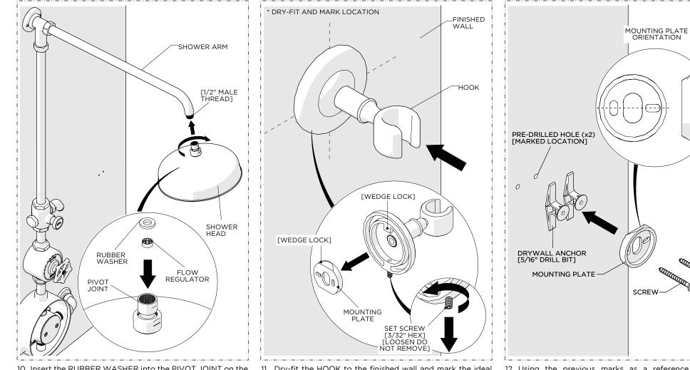
10. Insert the RUBBER WASHER into the PIVOT JOINT on the SHOWER HEAD (packaged separately) then thread and securely tighten the PIVOT JOINT onto the SHOWER ARM.
