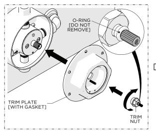
19. Slide the TRIM PLATE, in the desired orientation, over the ALL THREAD TUBE, then thread and securely tighten the TRIM NUT onto the TUBE.
