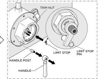
21. Remove the HANDLE and STEM then place the LIMIT STOP onto the TRIM NUT making sure it contacts with the LIMIT STOP PIN.
