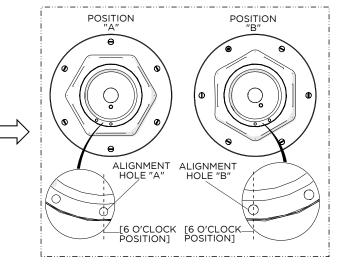
Determine the desired TRIM PLATE orientation and position the appropriate ALIGNMENT HOLE vertically at 6 o'clock.
