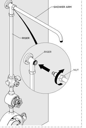
Insert the SHOWER ARM into the RISER then securely tighten the NUT.
