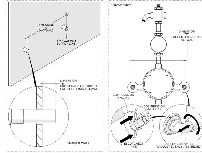
Measure the ACTUAL on-center spread (DIMENSION C) of the SUPPLY LINES, which MUST be between 12-3/4" [324mm] and 13-3/8" [340mm].
