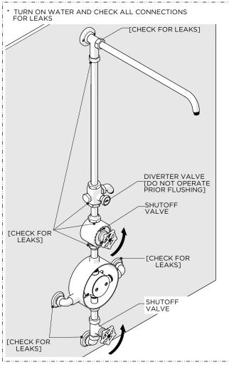
Turn on the water and operate the SHUTOFF VALVES to FLUSH out the supply lines, check all connections for leaks then turn the water off.
