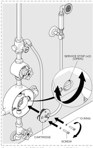
Install the CARTRIDGE using the SCREWS provided, making sure the O-RINGS are in place, then open the integrated SERVICE STOPS.
