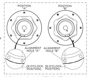
Determine the desired TRIM PLATE orientation and position the appropriate ALIGNMENT HOLE vertically at 6 o'clock.
