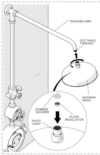
10. Insert the RUBBER WASHER into the PIVOT JOINT on the SHOWER HEAD (packaged separately) then thread and securely tighten the PIVOT JOINT onto the SHOWER ARM
