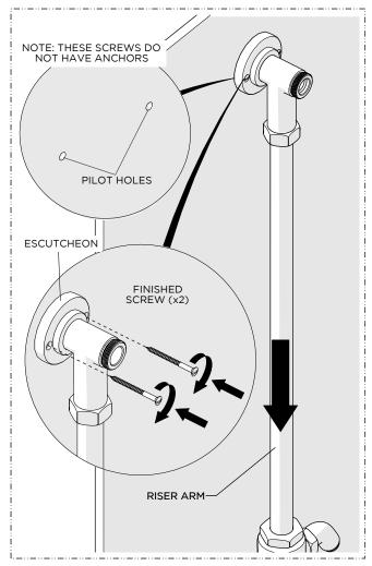
Remove the RISER TUBE then, using the previous marks, pre-drill the holes (pilot holes) to accommodate the 2-1/2" FINISHED WOOD SCREWS (x2) provided.
