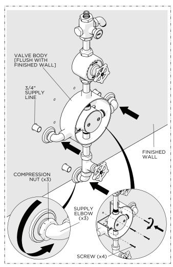
Fit the SUPPLY ELBOWS back onto the SUPPLY LINES making sure the VALVE BODY sits FLUSH against the finished wall and secure the VALVE BODY to the wall using the WOOD SCREWS (x4) provided then thread and securely tighten the COMPRESSION NUTS onto the FI BOWS.
