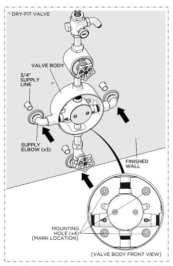
Fit the SUPPLY ELBOWS onto the SUPPLY LINES making sure the VALVE BODY sits flush against the finished wall then mark the location of the MOUNTING HOLES (x4).
