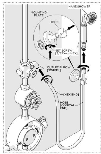
13. Place the HOOK onto the MOUNTING PLATE and securely tighten the SET SCREW then connect the HOSE to the HANDSHOWER and DIVERTER VALVE and place the HANSHOWER on the HOOK.
