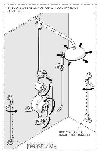
23. INSTALL THE SPRAY BARS PER THE INSTALLATION GUIDELINES PROVIDED WITH THE BARS THEN:
