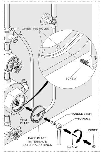
22. Align the SET SCREW on the back of the FACEPLATE with the ALIGNMENT HOLE at 6 o'clock on the TRIM PLATE then push the FACEPLATE into the TRIM PLATE making sure it is fully seated.
