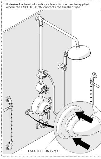
24. Slide the ESCUTCHEONS (x2) on the INLET ELBOWS against the finished wall.
