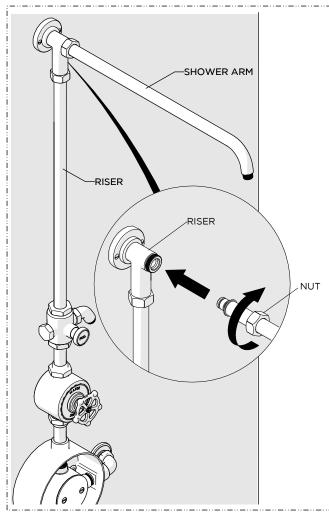
8. Insert the SHOWER ARM into the RISER then securely tighten the NUT.
