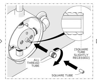
17. **FULLY** thread the ALL THREAD TUBE onto the CARTRDIGE then insert the SQUARE TUBE into the ALL THREAD and onto the CARTRIDGE STEM.
