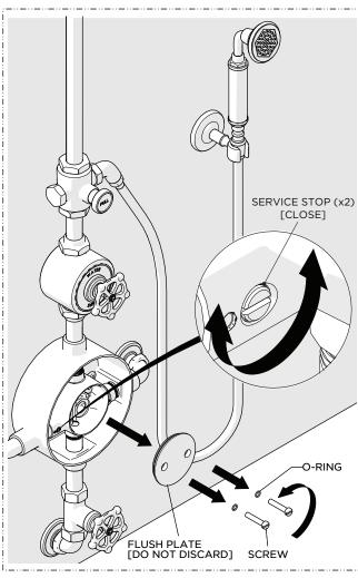
14. Close the integrated SERVICE STOPS on the VALVE then remove the FLUSH PLATE.
