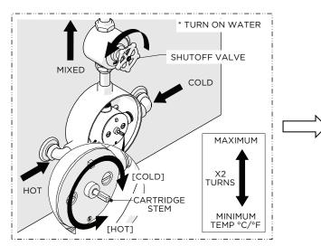
16. Turn on the water and open the SHUTOFF VALVE then slowly rotate the CARTRIDGE STEM clockwise to attain full cold then counterclockwise to attain full hot. It's approximately 2 complete rotations. Verify a full range of temperatures exists.
