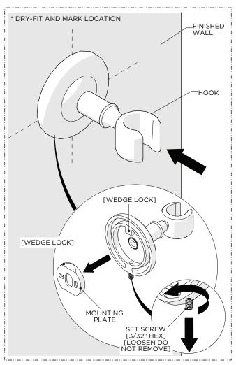
Dry-fit the HOOK to the finished wall and mark the ideal location for installation; preferably over adequate blocking or stud material.
