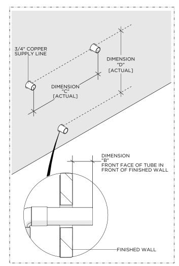
Measure the ACTUAL on-center spreads of the SUPPLY LINES:
