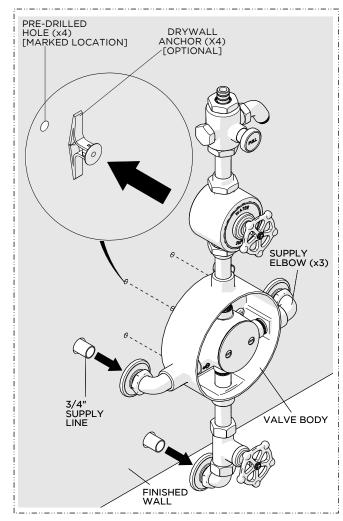
Remove the VALVE then, using the previous marks, predrill the holes (pilot holes) to accommodate the 1-1/2" WOOD SCREWS and, if necessary, install the DRYWALL ANCHORS provided where blocking is not installed.
