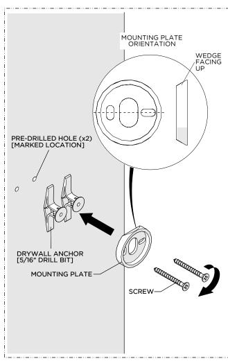
12. Using the previous marks as a reference, install the MOUNTING PLATE, using the ANCHORS (if needed) and WOOD SCREWS provided.
