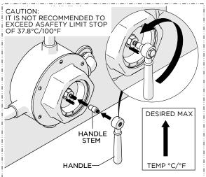
20. With water running, and using the HANDLE STEM and HANDLE adjust the temperature to the <u>MAXIMUM</u> desired bathing temperature, verified with a thermometer. Turn the water off and make sure **NOT** to change this setting.
