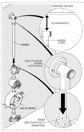
Fully insert the RISER TUBE into the top of the DIVERTER VALVE making sure the ESCUTCHEON for the SUPPORT POST sits FLUSH against the finished wall.
