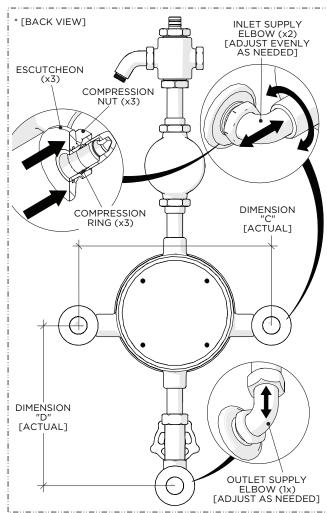
Push the ESCUTCHEONS against the COMPRESSION NUTS then measure the ACTUAL on-center spread of the INLET & OUTLET ELBOWS (DIMENSIONS C and D).
