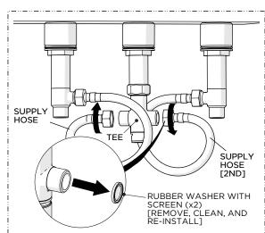
17. Turn off the water and unthread both the SUPPLY HOSES from the TEE to remove and clean the RUBBER WASHER WITH SCREENS then re-install the WASHERS and HOSES.
