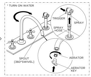
18. Re-install the AERATOR then turn on water and operate the SPRAY and SPOUT to ensure they operate and function properly.
