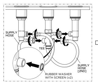
Connect the SIDEBODIES to the TEE using the SUPPLY HOSES provided. Securely tighten the HOSES and ensure they are not pinched/kinked.
