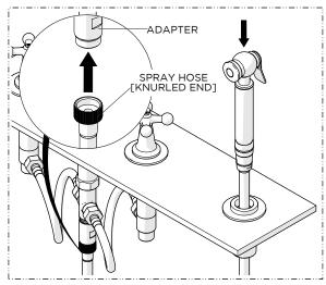
14. Insert the SPRAYER into the ESCUTCHEON until it stops then securely tighten the HOSE [knurled end] onto the TEE.
