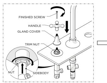
Re-attach the GLAND COVER, HANDLE and FINISHED SCREW. Ensure the HANDLE is in the desired orientation then securely tighten the NUT on the SIDEBODY.
