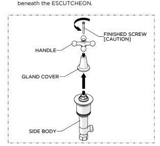
4. Carefully unthread the FINISHED SCREW then pull the HANDLE and the GLAND COVER up.
