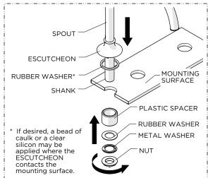
Insert the SPOUT through the hole on the mounting surface making sure the RUBBER WASHER provided is beneath the ESCUTCHEON then reinstall the PLASTIC SPACER, WASHERS and securely tighten the NUT.
