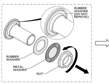
11. Unthread and remove the NUT, METAL WASHER, and RUBBER WASHER from the SHANK.
