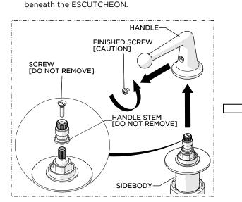
Carefully unthread the FINISHED SCREW then pull the HANDLE up.
