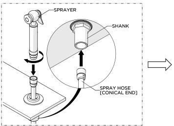
13. Insert the SPRAY HOSE [conical end] through the SHANK and the ESCUTHCHEON then thread and securely tighten the SPARYER onto the HOSE.
