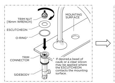
7. Place the ESCUTCHEON and O-RING over the TRIM CONNECTOR then thread and securely tighten the TRIM NUT into the TRIM CONNECTOR.
