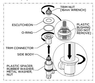
5. Unthread and remove the TRIM NUT, remove the ESCUTCHEON with the O-RING, unthread and remove the TRIM CONNECTOR then fully thread the NUT down the SIDEBODY.
