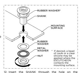
mounting surface making sure the RUBBER WASHER provided is beneath the ESCUTCHEON then re-install the WASHERS then securely tighten the NUT.
