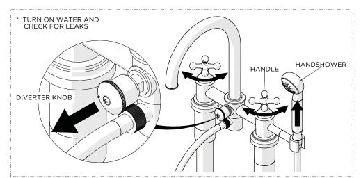
9. Turn on the water to flush out the supply lines, operate the HANDLES and DIVERTER KNOB to ensure they function properly, and carefully inspect all connections for leaks then turn off the water.
