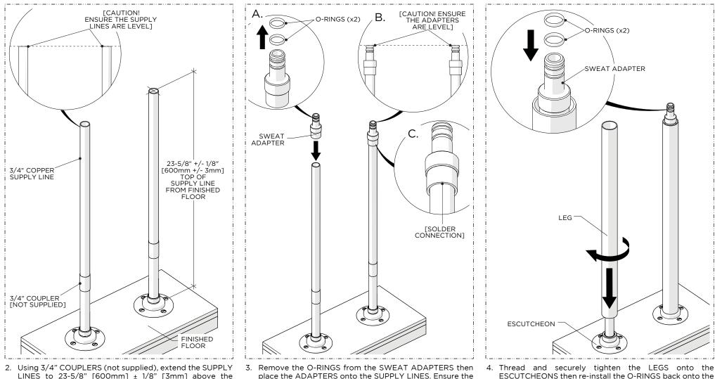
**IMPORTANT:** Ensure the SUPPLY LINES are level and free of any burrs.
