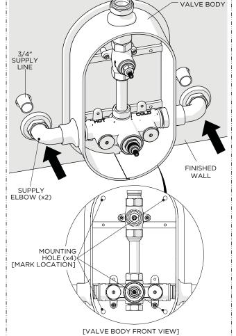
5. Fit the SUPPLY ELBOWS onto the SUPPLY LINES making sure the VALVE BODY sits flush against the finished wall then mark the location of the MOUNTING HOLES (x4).
