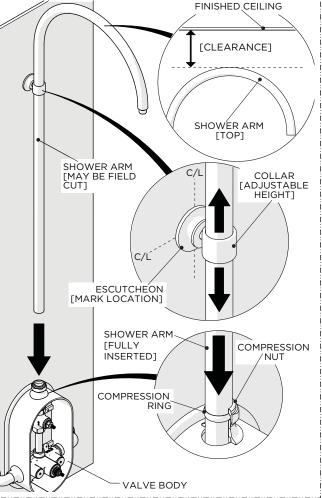
8. Fully insert the SHOWER ARM into the top of the VALVE BODY making sure the ESCUTCHEON for the SUPPORT POST sits flush against the finished wall and there is enough **clearance** between the top of the ARM and the finished ceiling.
