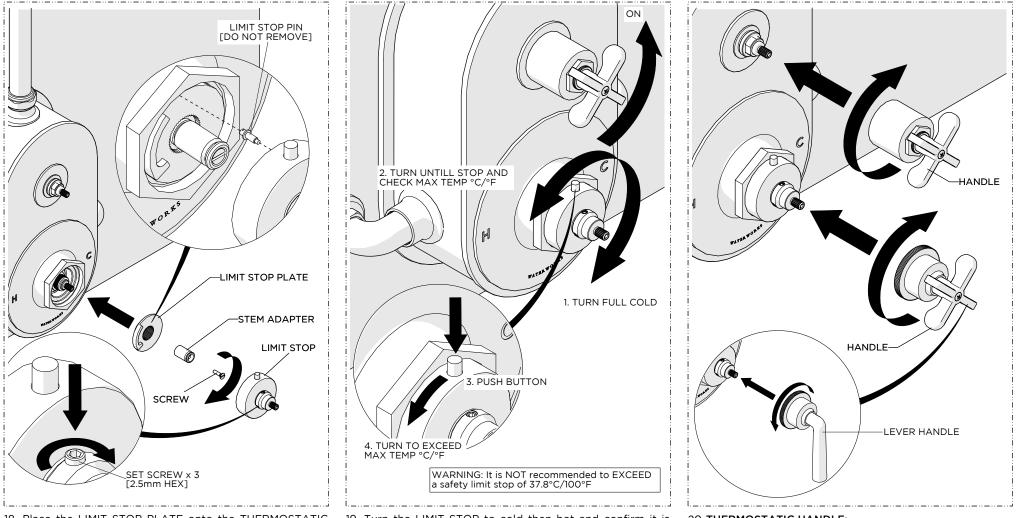
18. Place the LIMIT STOP PLATE onto the THERMOSTATIC VALVE in the desired orientation, place the STEM ADAPTER onto the CARTRIDGE and secure it using the SCREW provided.
