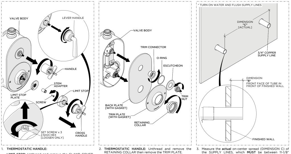
LIMIT STOP: Unthread and remove the GLAND COVER, loosen, but do NOT remove the SET SCREWS [2.5mm HEX], pull off the LIMIT STOP, unthread the SCREW, remove the STEM ADAPTER and LIMIT STOP PLATE.
