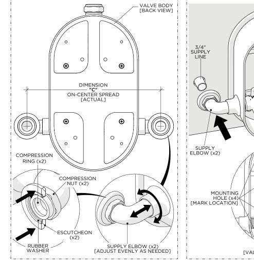
Push the ESCUTCHEONS against the COMPRESSION NUTS then measure the on-center spread of the SUPPLY ELBOWS (DIMENSION C).
