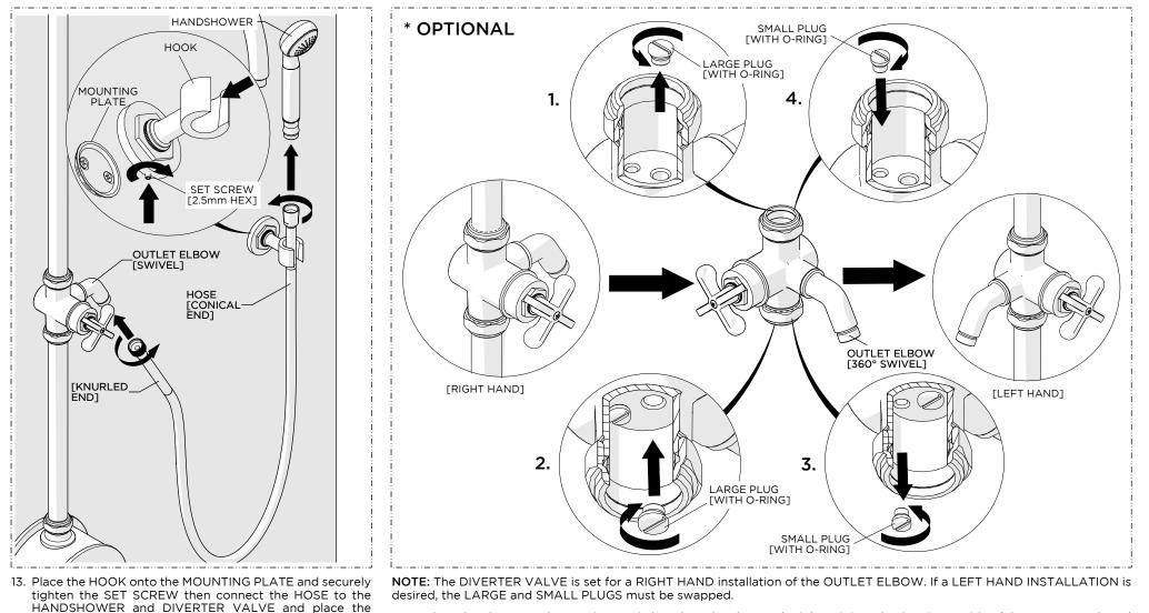
14. Unthread and remove the LARGE PLUG then thread and securely tighten it into the OPPOSITE side of the VALVE. Unthread and remove the SMALL PLUG then thread and securely tighten it into the OPPOSITE side of the VALVE. Ensure both PLUGS are securely tightened to prevent leaks then rotate the OUTLET ELBOW to the correct position.
