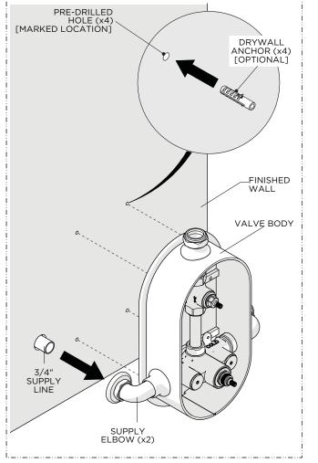
6. Remove the VALVE and, using the previous marks, predrill holes (pilot holes) to accommodate the MOUNTING SCREWS and, if necessary, install the DRYWALL ANCHORS provided where blocking is not installed.
