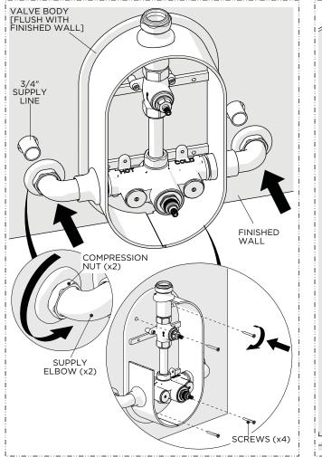
7. Fit the SUPPLY ELBOWS onto the SUPPLY LINES making sure the VALVE BODY sits **flush** against the finished wall and secure the VALVE BODY to the wall using the SCREWS (x4) provided then thread and securely tighten the COMPRESSION NUTS onto the ELBOWS.
