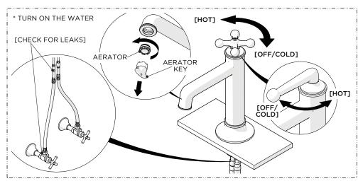
6. Unthread and remove the AERATOR from the SPOUT using the KEY provided then turn on the water and operate the HANDLE to ensure it functions properly and flush out any debris in the supply lines. Check all connections for leaks and turn off the water.
