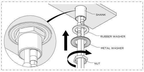
Re-attach the RUBBER and METAL WASHERS then thread and securely tighten the NUT onto the SHANK.
