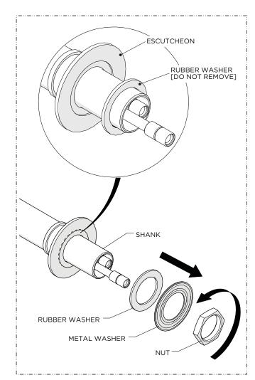
1. Unthread and remove the NUT from the SHANK then remove the METAL and RUBBER WASHERS
