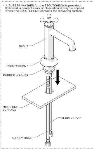
3. Insert the SPOUT through the hole on the mounting surface making sure the RUBBER WASHER provided is beneath the ESCUTCHEON.
