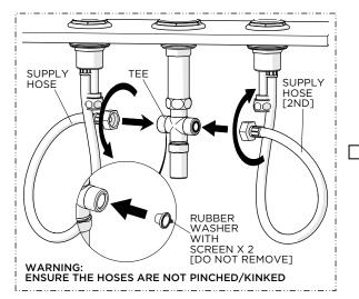
Thread and securely tighten the SUPPLY HOSES onto the TEE and ensure the HOSES are not pinched/kinked.
