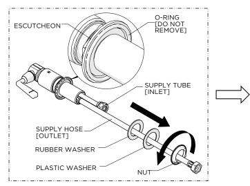
Unthread and remove the NUT from the HANDLE then remove the PLASTIC and RUBBER WASHERS.
