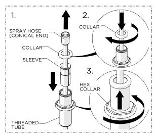
Insert the SPRAY HOSE through the THREADED TUBE, PLASTIC SLEEVE and COLLAR then insert the SLEEVE into the TUBE. Thread and securely tighten the COLLAR onto the TUBE then thread the HEX COLLAR until it stops.
