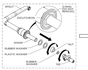
Unthread and remove the TEE and NUT from the SPOUT then remove the PLASTIC and RUBBER WASHERS.
