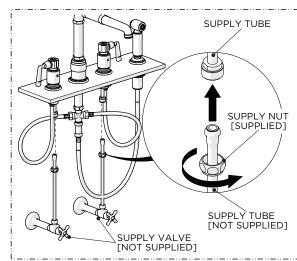
Unthread and remove the SUPPLY NUT from the SUPPLY TUBE, then make final SUPPLY VALVE [sold separately] connections.
