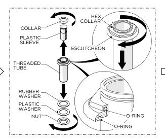
Unthread and remove the COLLAR, PLASTIC SLEEVE, NUT and WASHERS from the THREADED TUBE then partially unthread the HEX COLLAR.
