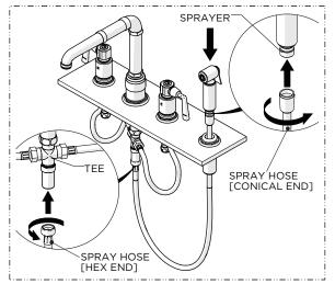
11. Thread and securely tighten the SPRAY HOSE [conical end] onto the SPRAYER and insert the HOSE into the PLASTIC SLEEVE until it stops then thread securely tighten the HOSE [hex end] onto the TEE.
