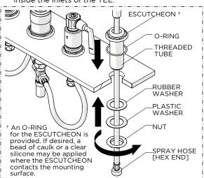
10. Insert the HOSE and THREADED TUBE through the hole on the mounting surface making sure the O-RING provided is beneath the ESCUTCHEON then re-install the WASHERS and NUT. Ensure the HEX COLLAR is properly aligned then securely tighten the NUT.
