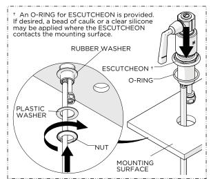
Insert the HANDLE through the hole on the mounting surface making sure the O-RING provided is beneath the ESCUTCHEON then reinstall the WASHERS and NUT. Ensure the HANDLE is properly aligned then securely tighten the NUT.
