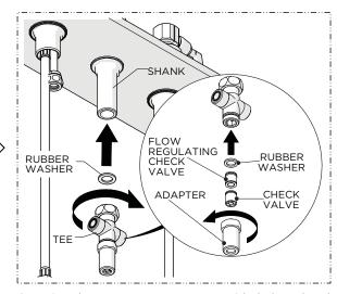
Using the RUBBER WASHER provided, thread and securely tighten the TEE back onto the SPOUT.
