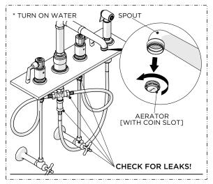
Remove the AERATOR then turn on the water to flush out any debris in the supply and inspect all connections for leaks.
