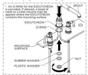
Insert the SPOUT through the hole on the mounting surface making sure the O-RING provided is beneath the ESCUTCHEON then re-install the WASHERS and NUT. Ensure the SPOUT is properly aligned then securely tighten the NUT.
