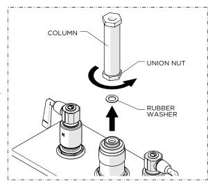
Unthread the UNION NUT then pull off the SPOUT COLUMN.
