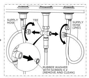
14. Turn off the water and unthread both the SUPPLY HOSES from the TEE to remove and clean the RUBBER WASHERS WITH SCREENS then re-install the WASHERS and HOSES.
