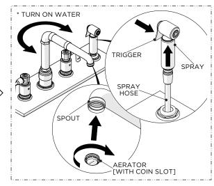
15. Re-install the AERATOR then turn on the water and operate the SPRAY to ensure it operates and functions properly and rotate the SPOUT to ensure it swivels properly.
