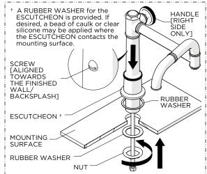
Insert the SPOUT through the hole on the mounting surface making sure the SCREW on the SPOUT COLUMN is aligned towards the finished wall then using the RUBBER WASHER provided thread and securely tighten the NUT onto the SHANK.
