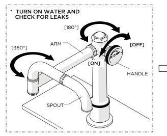
Turn on water and operate HANDLE and SPOUT to ensure they function properly and to flush out any debris in the supply line then check all connections for leaks and turn off the water.
