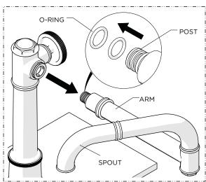
2. Remove the ARM to expose the POST and access the O-RINGS.
