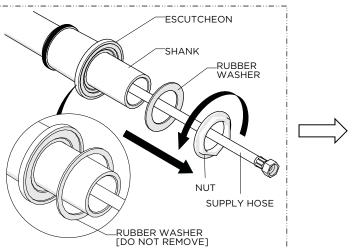
Unthread and remove the NUT and RUBBER WASHER from the SHANK.
