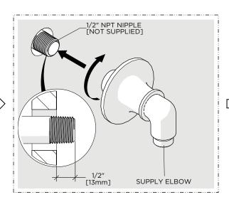
2. Ensure the 1/2" NPT NIPPLE (not supplied) projects 1/2" [13mm] from the surface of the finished wall then thread and securely tighten the SUPPLY ELBOW onto the NIPPLE.
