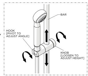
9. Place the HANDSHOWER on the HOOK and adjust the height and angle as needed.
