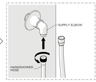
Thread and securely tighten the knurled end of the HOSE to the ELBOW.
