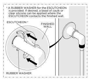
10. Slide the ESCUTCHEON up the ELBOW until it contacts the finished wall.
