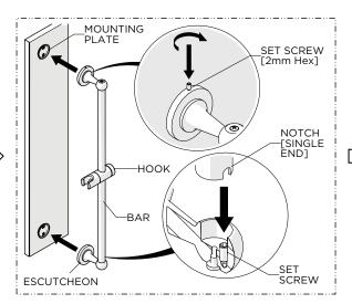
Place the BAR assembly over the MOUNTING PLATES, making sure the notch on the BAR is seated properly, then thread and securely tighten the SET SCREWS on each ESCUTCHEON.
