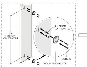
Install the MOUNTING PLATES at the proper oncenter spread of 24" [610mm] using the SCREWS provided.
