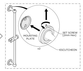
Loosen the SET SCREW on each ESCUTCHEON on the BAR using a 2mm HEX KEY and remove the MOUNTING PLATES.
