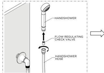
8. Thread and securely tighten the conical end of the HOSE to the HANDSHOWER.
