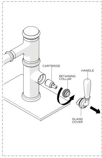
Remove the HANDLE then unthread and remove the RETAINING COLLAR to exposed and remove the CARTRIDGE.
