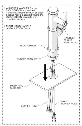
Insert the SPOUT through the hole on the mounting surface making sure the RUBBER WASHER provided is beneath the ESCUTCHEON and the HANDLE is aligned on the RIGHT SIDE of the SPOUT.
