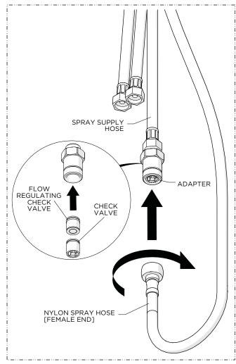
Thread and securely tighten the FEMALE END of the NYLON SPRAY HOSE onto SPRAY SUPPLY HOSE using the ADAPTER provided.
