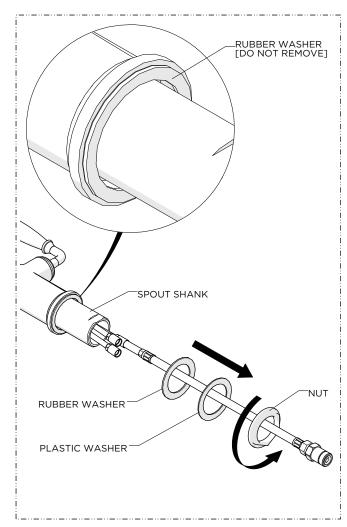
1. Unthread and remove the NUT from the SPOUT SHANK then remove the PLASTIC and RUBBER WASHERS.
