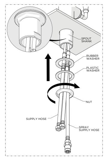
4. Slide the WASHERS and NUT over the HOSES then thread and securely tighten the NUT onto the SPOUT SHANK.
