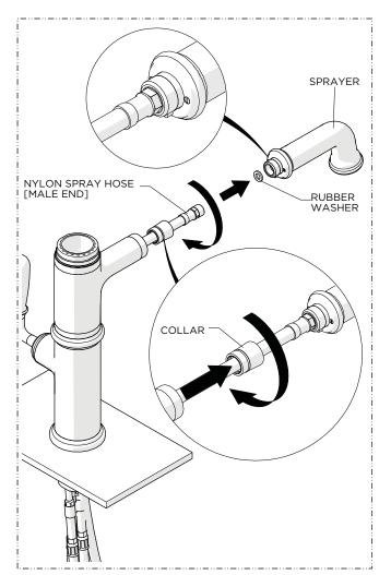
10. Thread and securely tighten the SPRAY HOSE into the SPRAYER using the RUBBER WASHER provided then thread and securely tighten the COLLAR back onto the SPRAYER.
