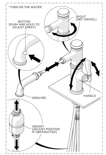
13. Turn on the water and operate the SPRAYER to ensure it functions properly making sure the WEIGHT can move freely beneath the cabinet and the SPOUT is able to swivel properly. Adjust the position of the WEIGHT if necessary.
