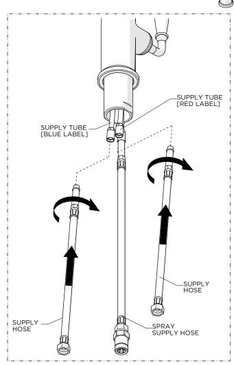
2. Thread and securely tighten the SUPPLY HOSES onto the SUPPLY TUBES pre-installed on the SPOUT.
