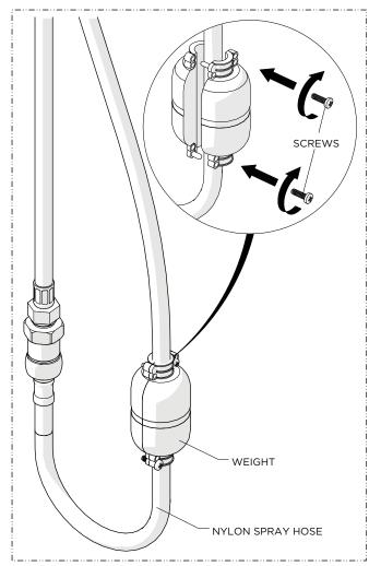
12. Align and press the two halves of the WEIGHT over the SPRAY HOSE in the desired position then thread and securely tighten the SCREWS provided.
