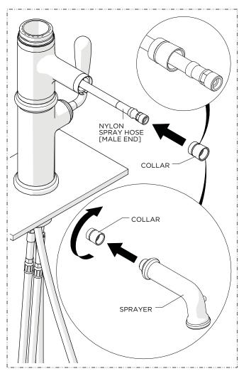
9. Unthread and remove the COLLAR from the SPRAYER inlet then slide the COLLAR over the SPRAY HOSE.
