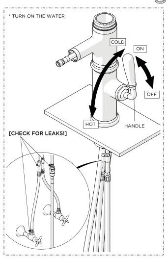
8. Turn on the water and operate the HANDLE to ensure it functions properly and to flush out any debris in the supply lines then check all connections for leaks and turn off the water.
