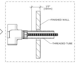
2. Mark the THREADED TUBE 1/2" [13mm] behind the finished wall.
