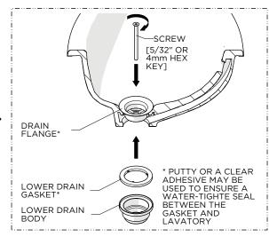
18. Re-install the LOWER DRAIN BODY making sure to use the GASKET provided. Ensure the GASKET makes a full seal on the underside of the lavatory then securely tighten the SCREW.
