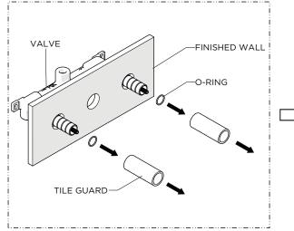
Remove the TILE GUARDS and the O-RINGS from the VALVE.
