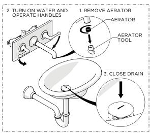
21. Removed the AERATOR, turn on the water to flush out the supply lines, and inspect all connections for leaks. Close the DRAIN to ensure it functions properly then turn off the water and re-install the AERATOR.
