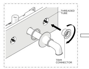
10. Thread and securely tighten the TRIM CONNECTOR onto the THREADED TUBE.
