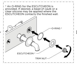
11. Hold the ESCUTCHEON against the finished wall, making sure to use the O-RING provided, and thread the TRIM NUT into TRIM CONNECTOR and securely tighten using a 5/8" [16mm] wrench.
