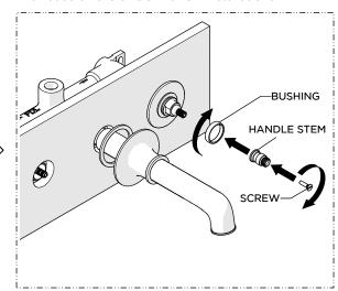
12. Thread the BUSHING onto the TRIM NUT. Place the HANDLE STEM onto the TRIM NUT then thread and securely tighten the SCREW.
