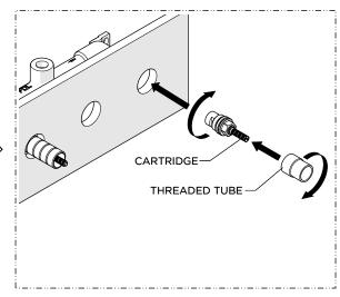
Thread and securely tighten the CARTRIDGE back into the VALVE then thread the THREADED TUBE back onto the CARTRIDGE.
