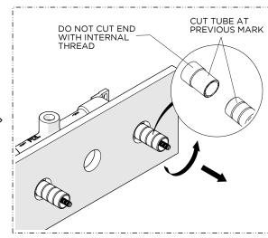
Unthread the THREADED TUBE then cut the TUBE at the previous mark. Do NOT cut the end with the internal thread.
