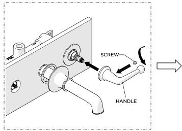
13. Place the HANDLE onto the HANDLE STEM in the desired orientation then thread and securely tighten the SCREW.
