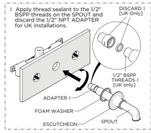
Apply thread sealant to the ADAPTER ‡ then thread and securely tighten the SPOUT into the VALVE.
