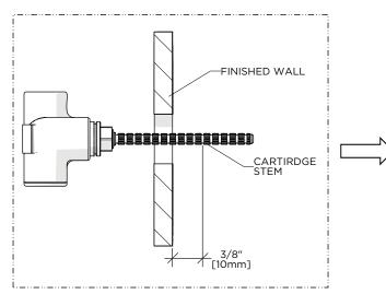
4. Mark the CARTRIDGE STEM 3/8" [10mm] beyond where it protrudes from the finished wall.
