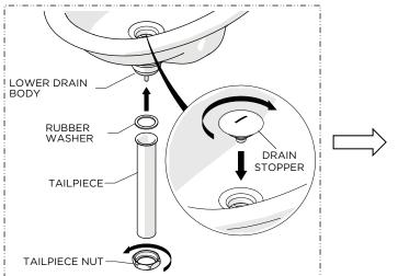
19. Re-install the DRAIN STOPPER then the TAILPIECE using the WASHER and NUT provided.
