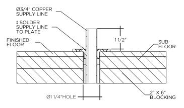
‡ DO NOT SOLDER COPPER PIPE UNTIL THE CORRECT ORIENTATION OF THE MOUNTING PLATE HAS BEEN DETERMINED
