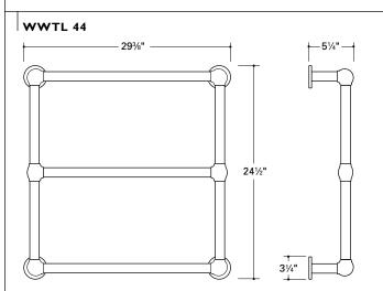
Note: 8' wire set exits from upper left-hand flange Electric: 115 volts (76 watts)
