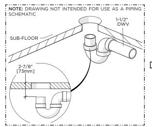
4. Rough-in a 1-1/2" DWV (not supplied). The top of the PIPE must be 2-7/8" [73mm] from the top of the sub-floor in order for the DRAIN HUB to be securely installed. Ensure all DWV pipes and fittings are well supported to eliminate the possibility of shifting.
