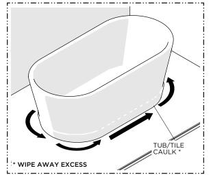
20. Run a bead of tub and tile caulk around the bottom edge of the BATHTUB where it meets the finished floor; wipe away any excess caulk with a wet paper towel.
