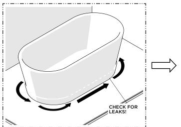
19. Drain the BATHTUB and check for leaks.
