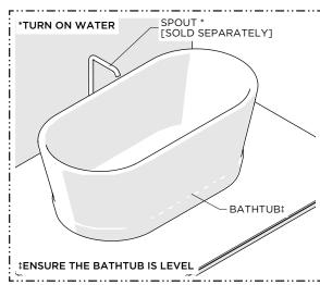
18. Verify the BATHTUB is level and, if needed, add shims then fill the BATHTUB making sure the DRAIN STOPPER functions properly.
