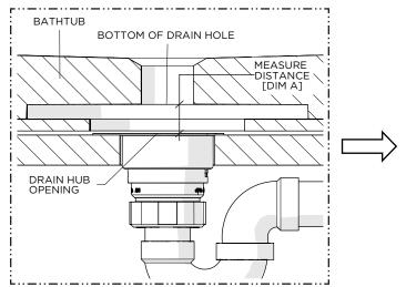
Measure the distance between the opening on the DRAIN HUB to the bottom of the BATHTUB drain hole.
