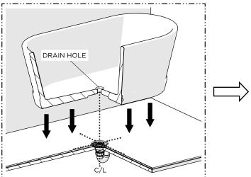
13. Move the BATHTUB into position with the DRAIN HOLE aligned with the TAILPIECE.
