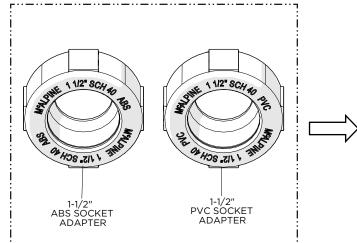
Select either the ABS or PVC SOCKET ADAPTER, depending on the material of the DWV piping.
