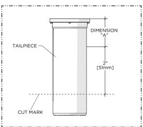
11. Add 2" [51mm] to the previous measurement (DIM A) taken and cut the TAILPIECE to that length.
