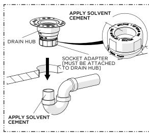
Apply the appropriate solvent cement to the inside of the SOCKET ADAPTER and the outside of the 1-1/2" DWV pipe then connect the ADAPTER to the pipe.
