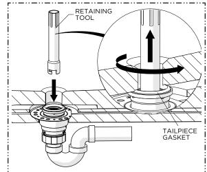
14. Insert the RETAINING TOOL into the TAILPIECE and rotate counterclockwise to engage the tabs inside the TAILPIECE and slots on the TOOL. Pull up so the TAILPIECE GASKET makes contact with the underside of the BATHTUB.
