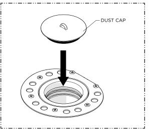
8. Insert the DUST CAP into the DRAIN HUB to protect the DRAIN during construction.
