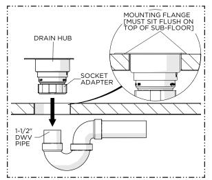
5. Dry-fit the the DRAIN HUB assembly to the 1-1/2" DWV pipe making sure the pipe fits snugly into the SOCKET ADAPTER and the MOUNTING FLANGE sits flush on top of the sub-floor.
