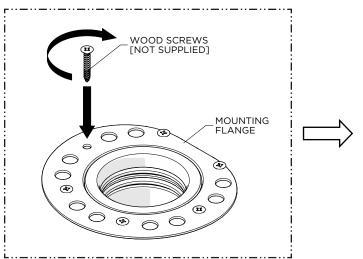
Secure the DRAIN HUB to the sub-floor using wood screws (not provided) through the small holes on the MOUNTING FLANGE.
