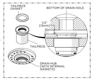
12. Insert the TAILPIECE into the DRAIN HUB. If necessary, lubricate the RUBBER GASKETS inside the HUB with some water or silicone grease. Make sure the TAILPIECE GASKET is in place on top of the TAILPIECE.
