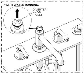
16. With water running, operate the DIVERTER KNOB to ensure it and the HANDSHOWER function properly.
