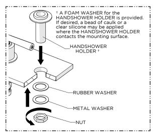
10. Insert the HANDSHOWER HOLDER through the hole on the mounting surface then re-install the WASHERS and securely tighten the NUT.
