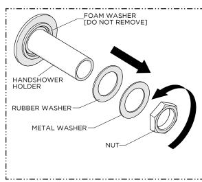
Remove the NUT, METAL WASHER, and RUBBER WASHER from the HANDSHOWER HOLDER.
