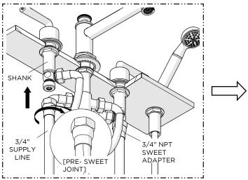
13. Pre-sweat 3/4" female NPT x sweat adapters to 3/4" supply lines and let cool. Apply a thin coat of pipe thread sealant to the male threads on the SHANKS then thread and securely tighten the ADAPTERS onto the SHANKS.
