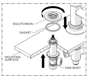
5. Using the GASKET provided, thread the ESCUTCHEON back onto the SIDEBODY until snug then let it rest on the mounting surface.
