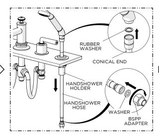
11. Using the RUBBER WASHER provided, thread the conical end of the HANDSHOWER HOSE into the HANDSHOWER then insert the other end of the HANDSHOWER HOSE through the HANDSHOWER HOLDER, then connect the open hose end to the BSPP ADAPTER along with the WASHER provided.
