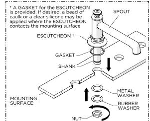
2. Insert the SHANK through the hole on the mounting surface, making sure the GASKET is beneath the ESCUTCHEON, then re-install the LOWER DECK WASHERS and securely tighten the NUT.
