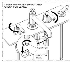
15. Remove the AERATOR using the TOOL provided then turn on the water supply and operate the HANDLES to flush out the supply lines and check all connections for leaks.
