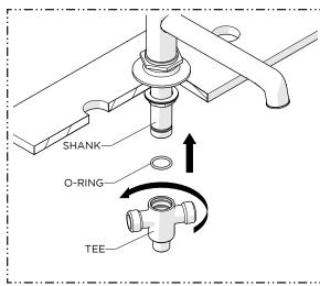
3. Thread and securely tighten the TEE onto the SHANK making sure to use the O-RING provided.
