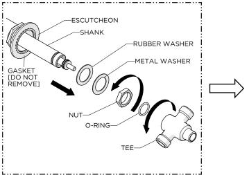
Remove the TEE, NUT and LOWER DECK WASHERS from the SPOUT SHANK.
