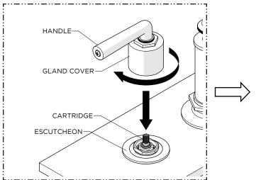
7. With the HANDLE in the required orientation, thread the GLAND COVER onto the ESCUTCHEON until snug.
