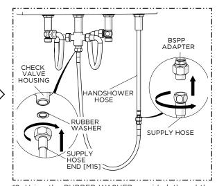
12. Using the RUBBER WASHER provided, thread the SUPPLY HOSE into the CHECK VALVE HOUSING then other end of the HOSE to BSPP ADAPTER in the HANDSHOWER HOSE.
