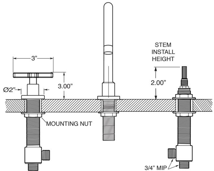
Spout and valves install through 1-1/4" diameter holes.
