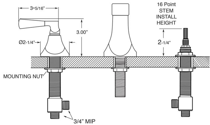
NOTE: Spout and valves install through 1-1/4" diameter holes. Plumber to provide 3/4" supply lines to valves
