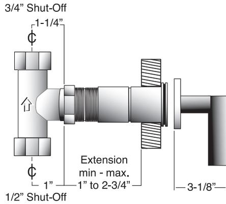
**Caution:** Minimalist design requirements create demanding installation. Read carefully. Cut and install all parts as level and straight as possible.
