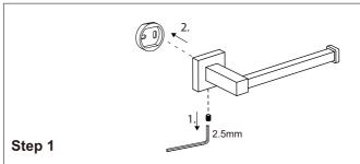
Loosen the set screw on the accessory and remove the backing plate. Position the accessory against the wall and mark outline with pencil.
