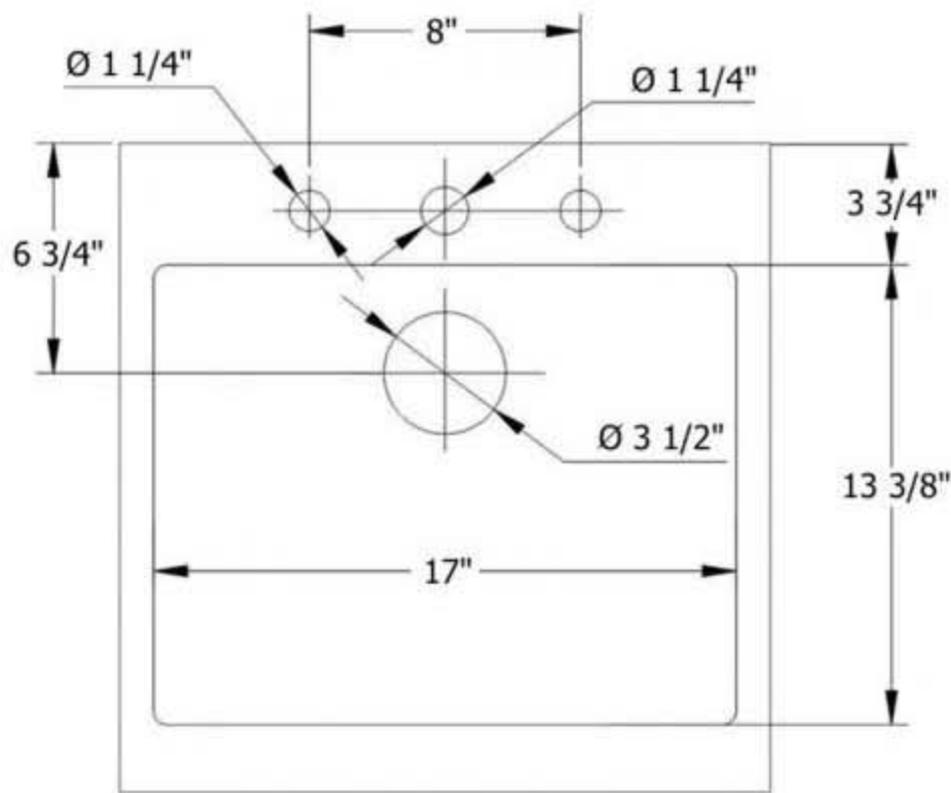
Note: Due to the nature of Fireclay, variations of up to 1/4" in size can occur. Cabinets and/or countertops should be cut to actual sink measurements after sink is on site.
