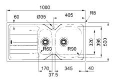
Reversible 1.5 bowl, single drainer with single drainer complete with 1 tap hole. Bright drainer/matt bowl. Made from 0.6 mm stainless steel.
