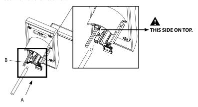
**Step 2:** Position the Outside Trim Plate Assembly through the bore hole.
