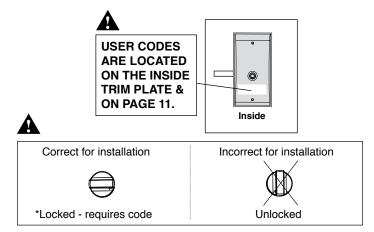
\*Locked position is required for installation and removal of the Inside Trim Plate Assembly. (Does not apply to Keypad Storeroom/Gate product)
