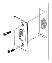
**Step 2:** Fasten Latch using two #8 x ¾" Wood Screws (item #6).
